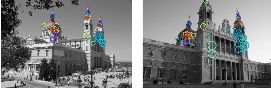
Fig. 1. Learned local features and descriptors matched with ASMK. Features assigned to the same visual word (65k words codebook) are shown in the same color; only top 20 common visual words (out of 94) are included. Accurate localization is not required since we do not use spatial verification to perform instance-level recognition.
