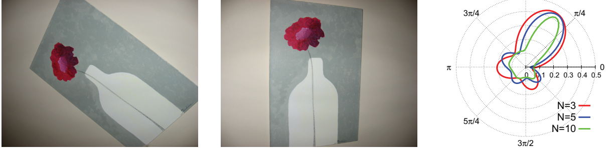
Fig. 4. Matching example of two images and similarity estimation for all possible image rotations. The image on the left undergoes rotation. Image similarity versus rotation is shown in polar coordinates, with the angular direction corresponding to the image rotation, and the radial to the image similarity score. This example is computed with angular modulation of VLAD, while using 3, 5 or 10 frequencies.
