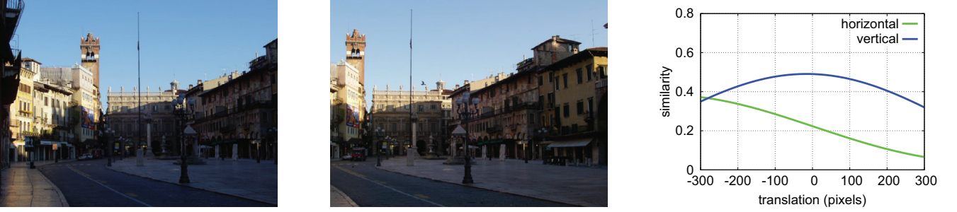
Fig. 6. Matching example of two images and similarity estimation for all possible image translations. Image on the left undergoes translation independently to the horizontal and the vertical direction. Modulated VLAD is used for the example.
