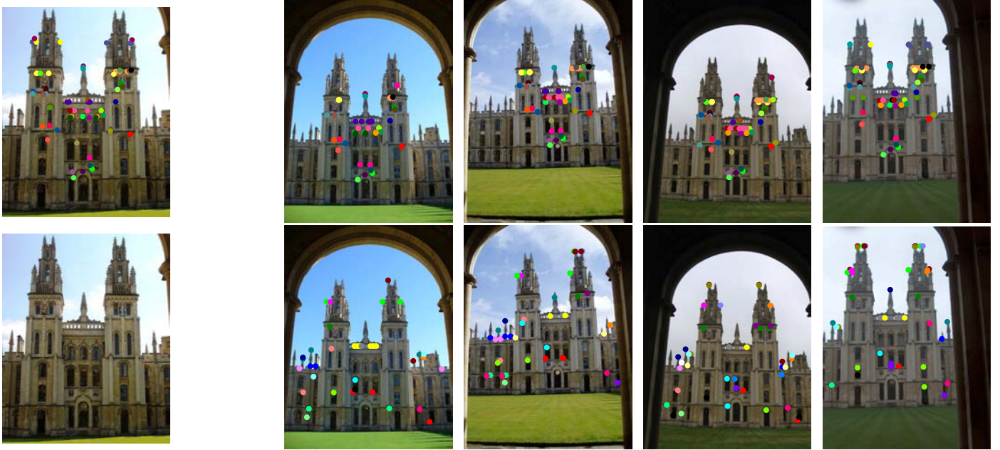
Figure 4: Sample reliable images and features assigned to reliable visual words, when geometry is not used. Left : Query image. Top : Features assigned to reliable visual words that appear in the query image. Bottom : Features in the set of augmented visual words. Note: we only show a subsample of the actual reliable visual words. Each color represents a distinct visual word.
