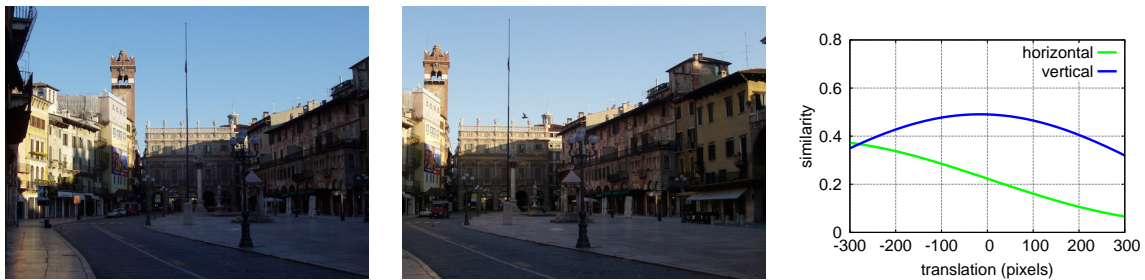
Figure 12: Matching example of two images and similarity estimation for all possible image translations. Image on the left undergoes translation independently to the horizontal and the vertical direction. VLAD jointly encoded with 2D coordinates of the local features is used for the example.
