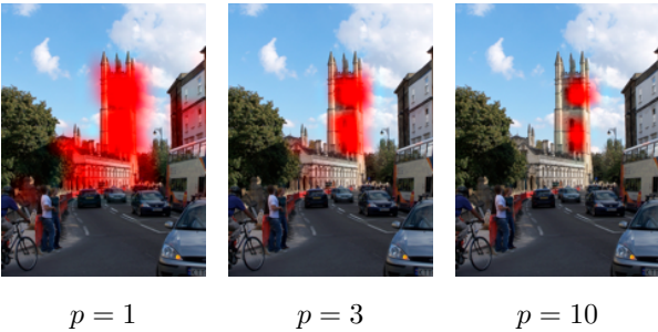
Fig. 4. Visualization of \mathcal{X}_k^p projected on the original image for three different values of p . Case p = 1 corresponds to SPoC, and larger p corresponds to GeM before the summation of (3). Examples shown use the off-the-shelf VGG.
