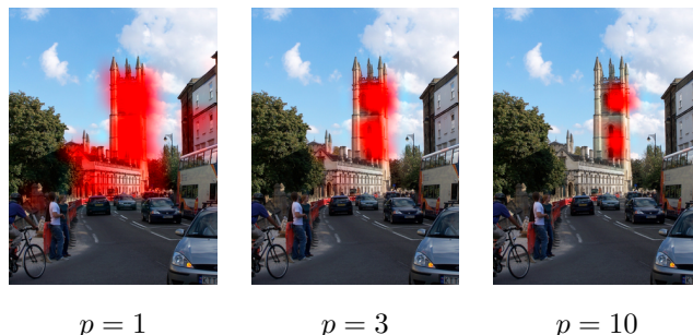
Figure 3: Visualization of feature map activations raised to the power of \alpha and then projected on the original image. Case p = 1 corresponds to SPoC, and larger p corresponds to GeM which becomes more localized.
