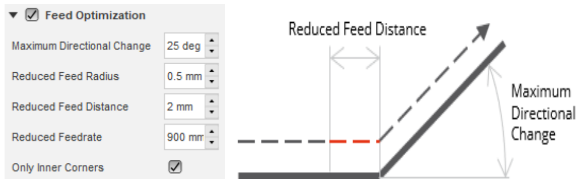
Figure 5 - Corner Feed Rate Reduction - Maximum directional change
