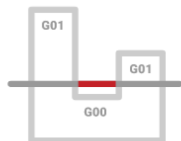
Figure 9 - Air Cuts reduction principle (Icam, 2010)
