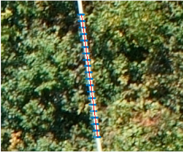
■ Figure 5.12 Transforming a set of Hough lines into a polyline by sampling points (blue) and fitting a RANSAC line (red).
