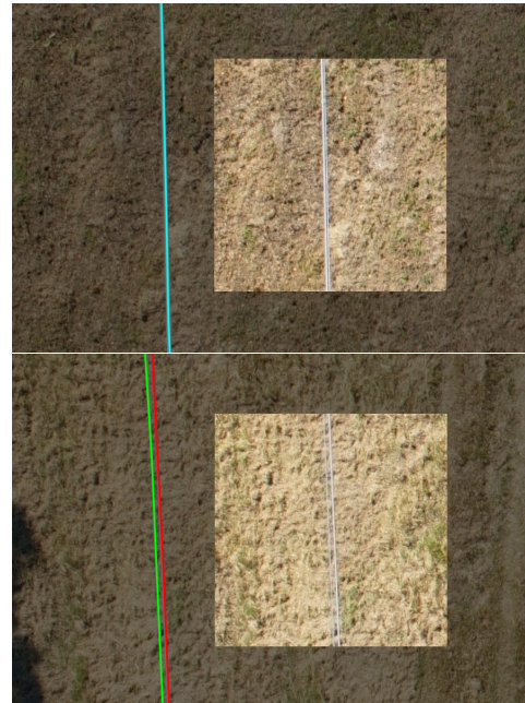
■ Figure 5.13 Example of unsuccessful (top) and successful (bottom) detection of two closely recorded wires.
