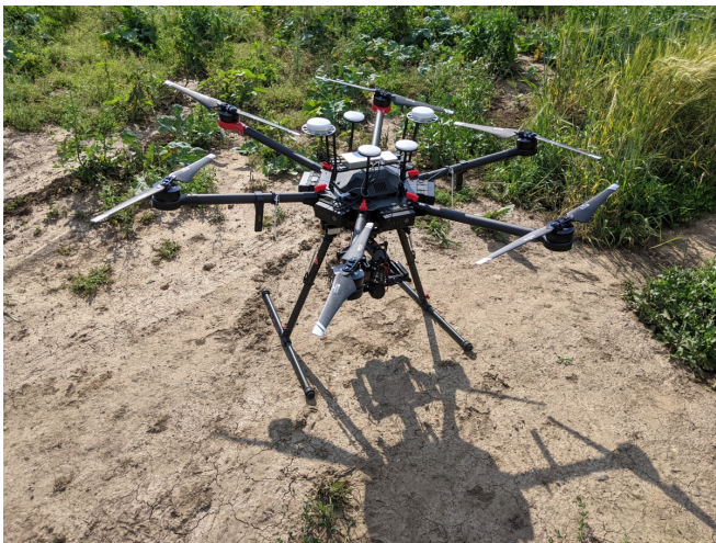
(a) DJI Matrice 600 hexa-rotor UAV with payload.
