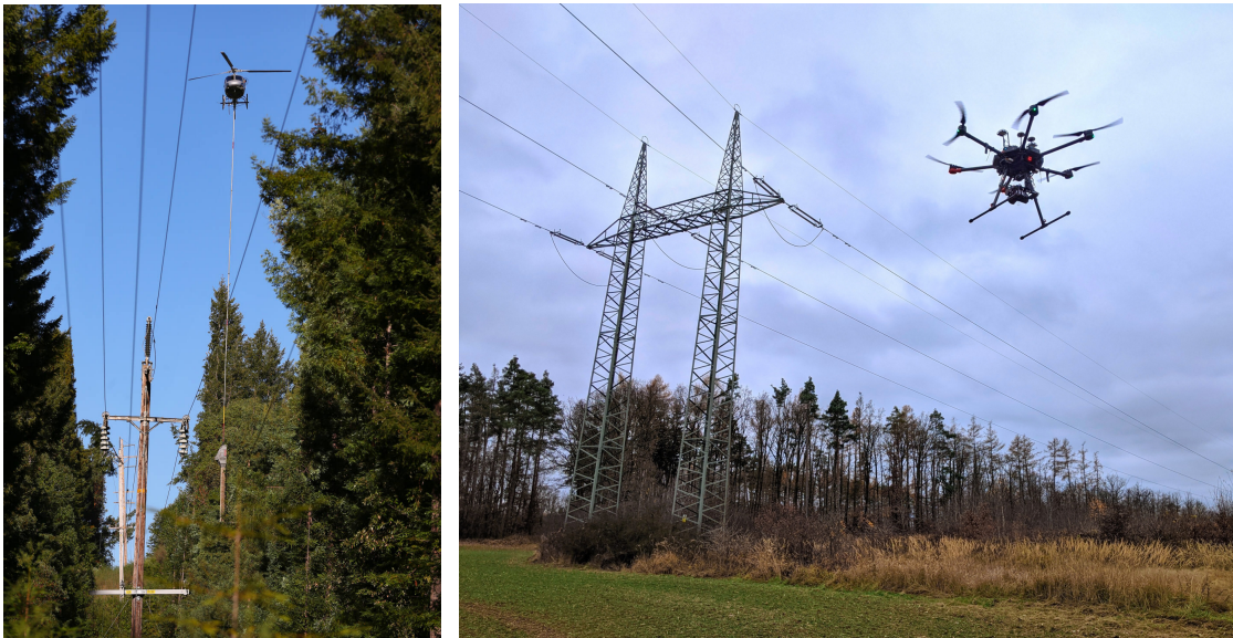
(a) Trimming vegetation using a big chainsaw hanging from a helicopter. (b) A multi-rotor UAV taking images of the power lines during our experiments.
