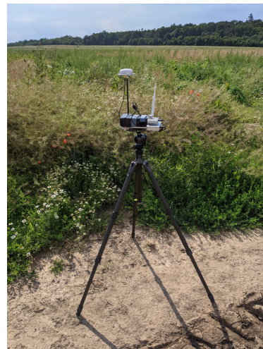
(b) DJI D-RTK GNSS mobile station.
