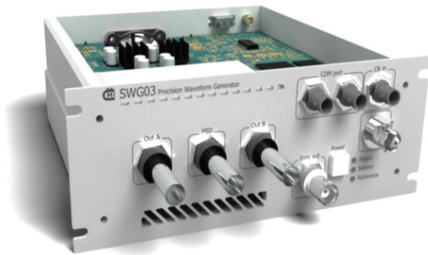
Fig. 4 Design of SWG generator. Voltage output of channel A and B together with center point-ground (left), optic fiber ports for control and external clock (right top), external voltage reference input (right middle), sync out and status LEDs (right bottom). Active air cooling of inner parts improves stability of output voltage under different loads.
