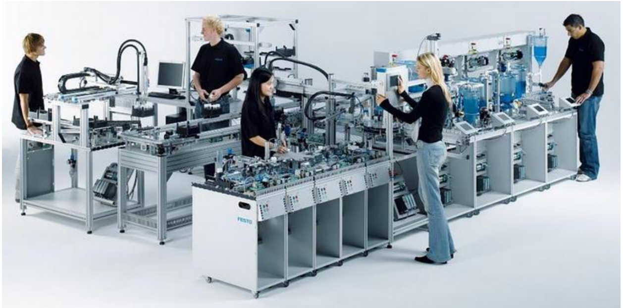
Figure 2: An example of flexible manufacturing systems developed by FESTO group [10]
