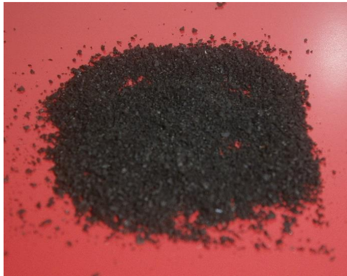
Figure 3.3 Crumb rubber modifier (30-40-mesh) reclaimed from old scrap tires
