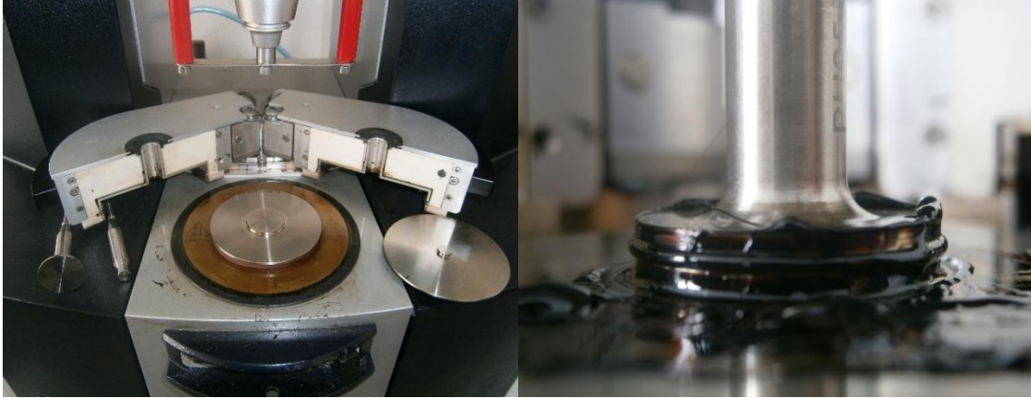
Figure 3.12 Dynamic shear rheometer (left) and a sample sandwiched between the two plates (right)
