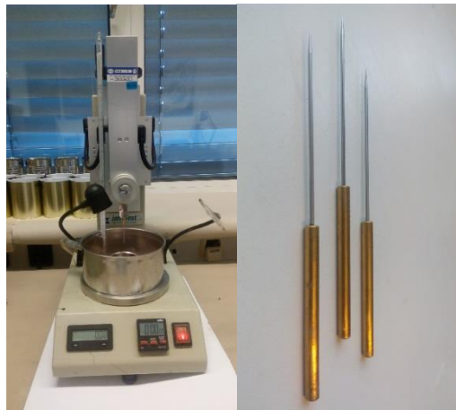
Figure 3.7 Penetrometer and the penetration needles
