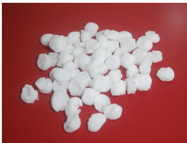
Figure 3.2 Free-flowing pellets of SBS modifier before high shear mixing
