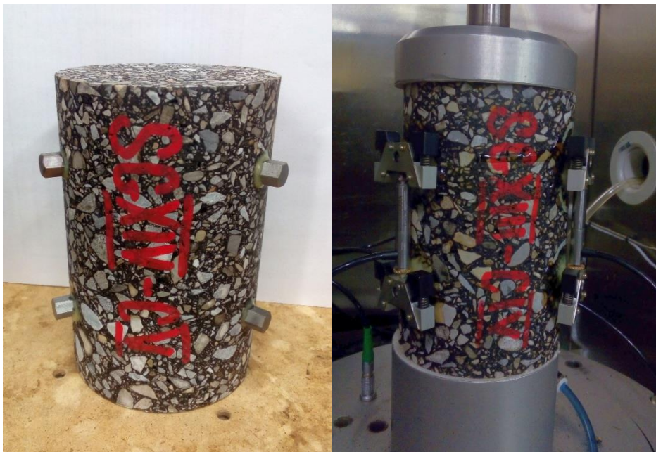
Figure 3.17 Dynamic modulus test specimen (left), LVDTs mounted to the specimen (right)
