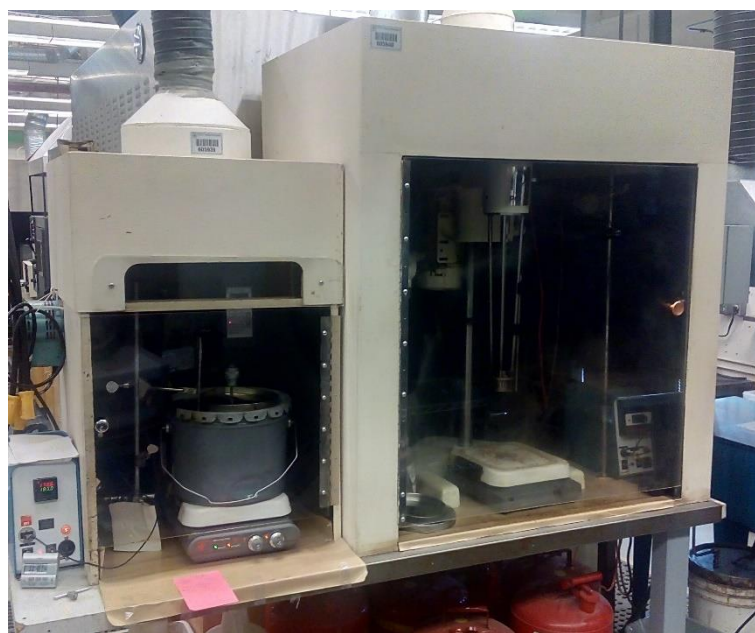
Figure 3.4 Low (left) and high shear (right) mixers used in the study
