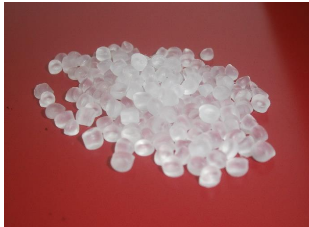
Figure 3.1 Free-flowing pellets of Elvaloy™ 5160 before low shear mixing with asphalt base
