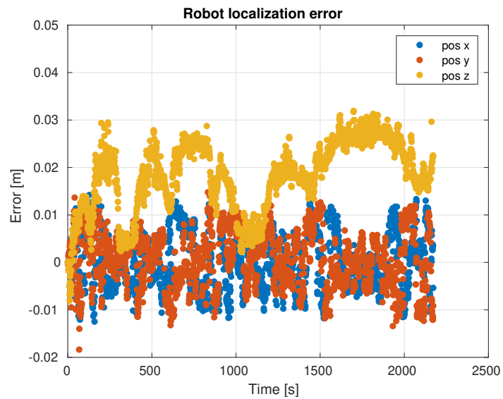
Figure 4.5: Robot estimated position error during the Naex 1 experiment.
