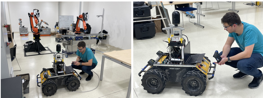
Figure 4.27: Photos from experiment in Testbed taken while the robot stood still and the terrestrial scanner was gathering data. The operator sat next to the robot and held the teleoperation controller.
