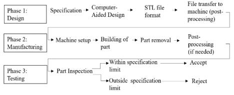
Fig. 1. Phases of Additive Manufacturing
