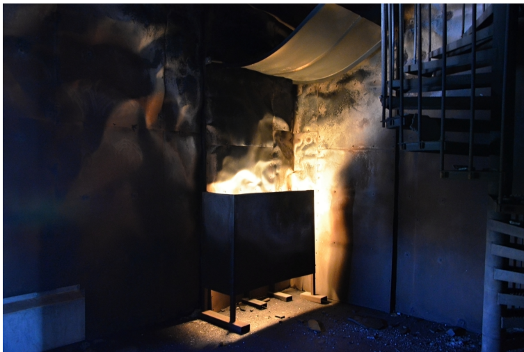
Figure 13: Example of fire test near spiral staircase in the first floor.
