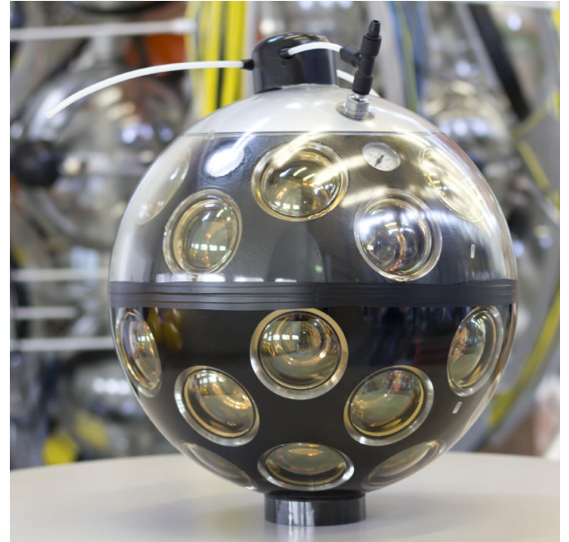
FIGURE 5. A prototype of the KM3NeT optical module. The components on the top are for the connection to the cable along the string. The metal structure inside the sphere serves for cooling purposes. Figure provided by the KM3NeT collaboration.
