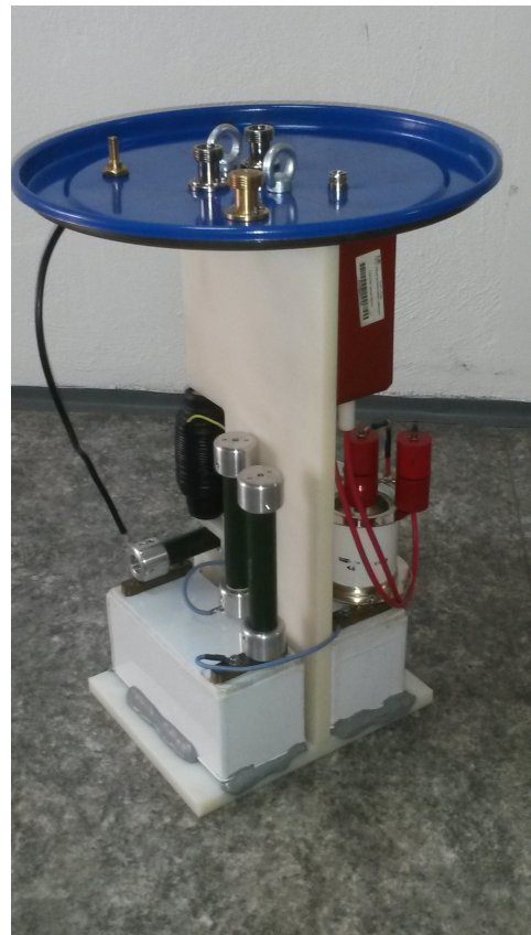
Figure 4.12: Photographs of the front and rear view of the charging circuit. While in operation, the circuit is enclosed in a barrel filled with biodegradable oil to isolate the circuit and avoid unwanted breakdowns.
