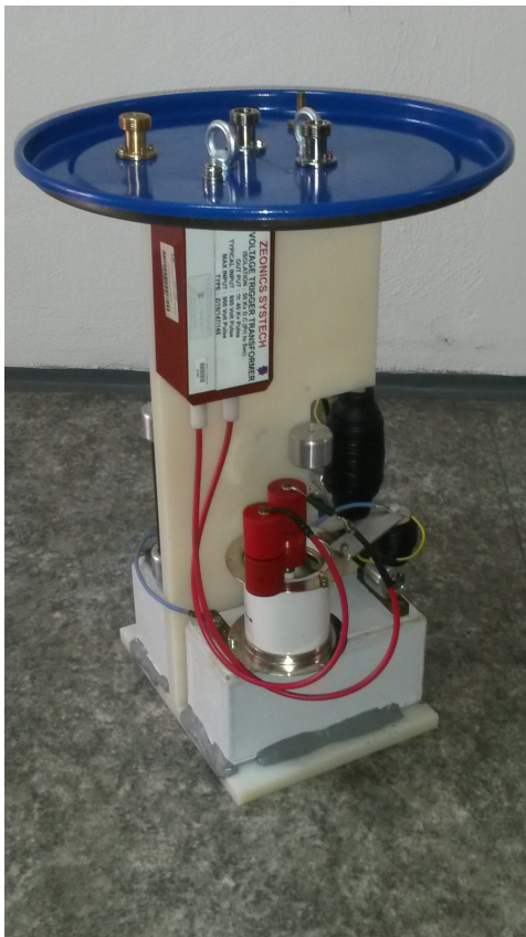
Figure 4.12: Photographs of the front and rear view of the charging circuit. While in operation, the circuit is enclosed in a barrel filled with biodegradable oil to isolate the circuit and avoid unwanted breakdowns.
