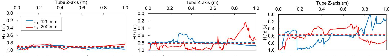
The dimensionless distance (mean value = dashed line) from the irradiated wall was comparable for geometrically similar tubes at the same flow regime. The hydrodynamic conditions based on the original CFD model for the tubes  $d_1$  are therefore also applicable to geometrically similar systems with a different scale.
