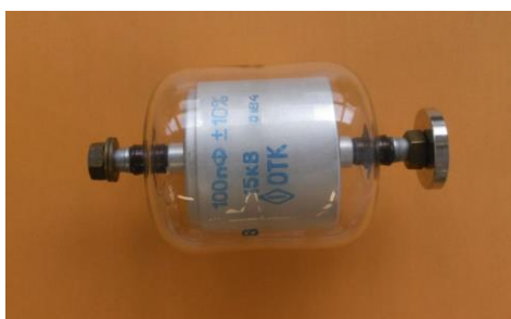
Figure 5: Vacuum capacitor used as an etalon.
