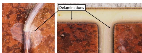
Fig. 9. Iodine Vapour Test results after 4 h at 80 °C
