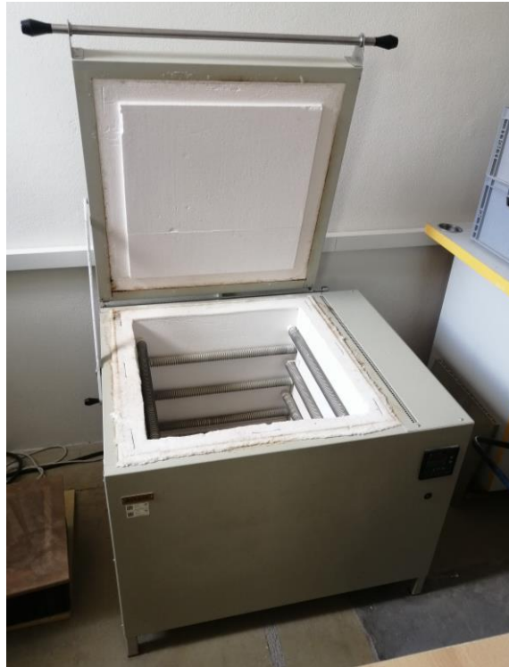
Fig. 3.10 Electric furnace 10013V.
