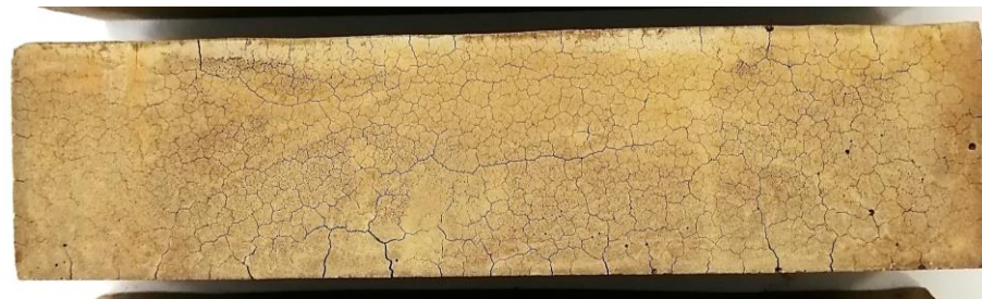
Fig. 4.8 Visible cracks on the specimen surface after heating to 400°C.
