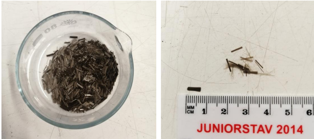
Fig. 3.3 Basalt fibers, with a diameter of 13 \mu\text{m} and a length of 6.35 mm.
