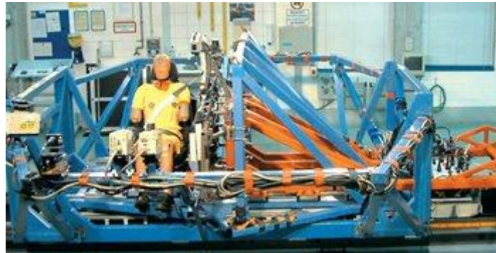
Figure 23: Continental sled setup safety [27]
