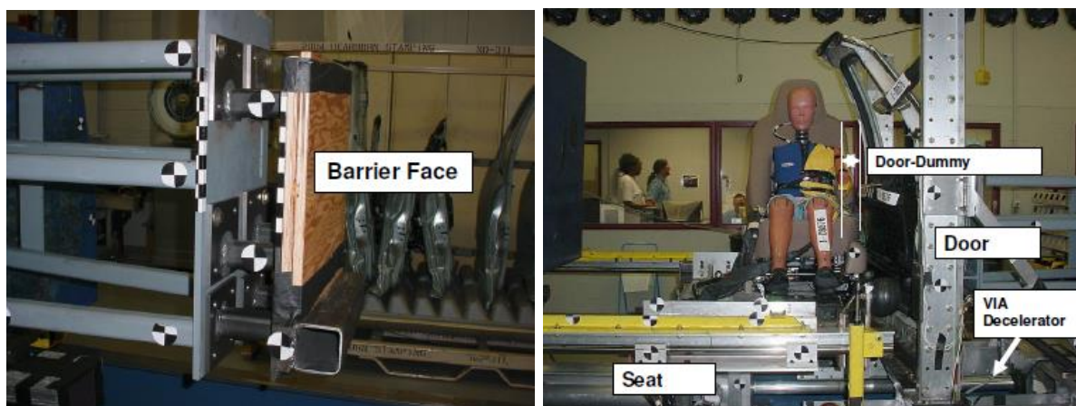
Figure 13: Barrier strike test setup as discussed in [16] – left: barrier face carriage; right – door and dummy carriage
