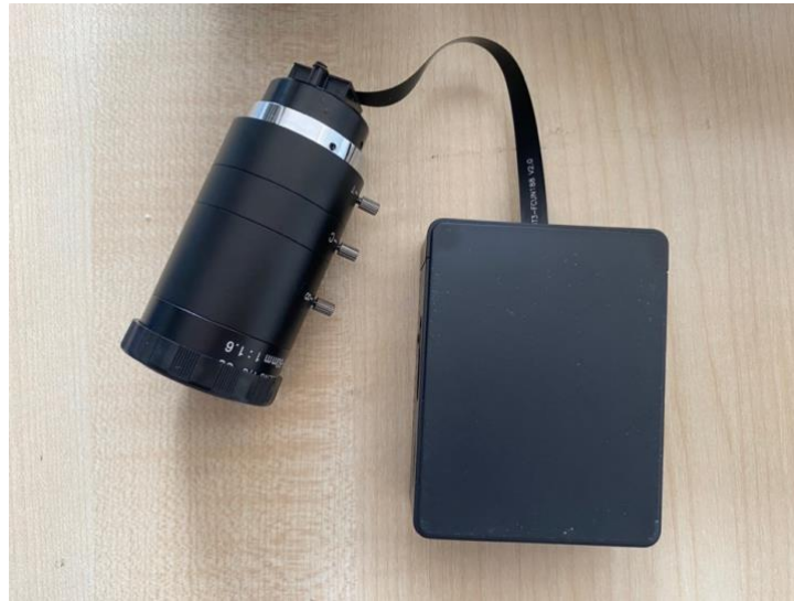
Figure 4.10: Integration of the CCTV lens and Attez WiFi camcorder [photo – author].
