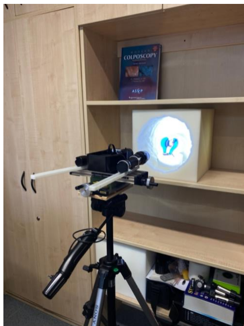
Figures 4.12: View of the simplified colposcope model being used on the phantom of the cervix [photo – author].
