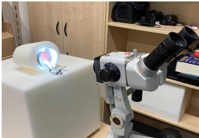
Figure 4.8: Karl Kaps colposcope KP3000 and view of the phantom model [photo – author].
