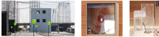
FIGURE 11. Photos of the MBZIRC 2020 Fire Challenge area. The photo on the left shows the tall structure simulating a building, the photo in the middle shows front view of the fire analogues (this unit was turned on) and the photo on the right shows side view of the fire analogues (this unit was turned off).
