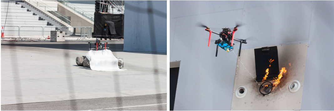
Figure 1.4: Photos from the firefighting challenge of the MBZIRC 2020 in Abu Dhabi, UAE. The left image shows fire extinguishing using a fire blanket. The right image displays UAV during the extinguishing of fire on the building facade by spraying a fire-extinguishing agent [14a], [18a].
