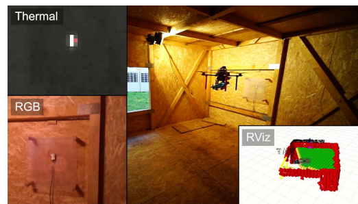
FIGURE 1. The proposed system uses processed data from the onboard sensors of the MAV towards the goal to extinguish fire inside the building.
