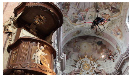
Fig. 1. Demonstration of the presented formation flying approach to realize a flying “film crew” in a church in Sternberk, Moravia.
