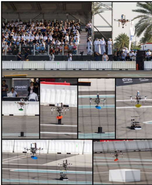
FIGURE 24 Photos from the MBZIRC competition. The upper image shows the UAV while following the static sweeping trajectory. The images in the middle row and the left on the lower part of the figure capture the moments when the UAVs were grasping objects. The remaining image shows an object being dropped into the dropping box. During four trials within the competition (two for Challenge 3 and two for the Grand Challenge), 25 objects overall were placed into the dropping zone (Table 3). http://mrs.felk.cvut.cz/jfr2018treasurehunt-video4 . MBZIRC: Mohamed Bin Zayed International Robotics Challenge; UAV: unmanned aerial vehicle [Color figure can be viewed at wileyonlinelibrary.com]
