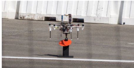
Photo of a UAV grasping a static object from the stand.
