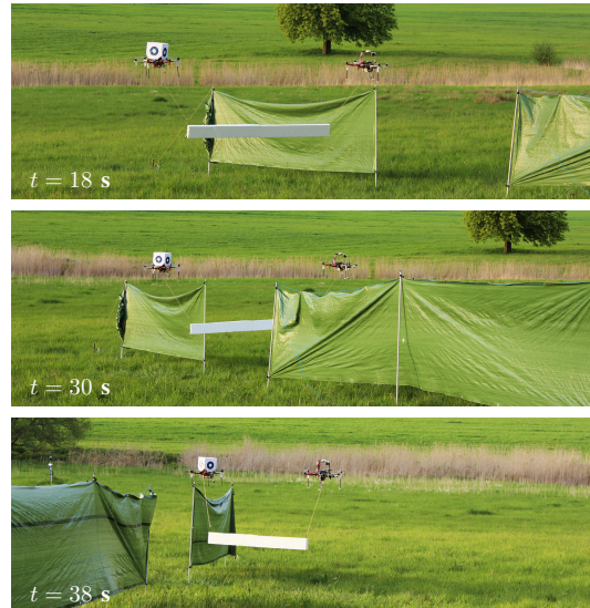
Fig. 6: Snapshots from the outdoor experiment, in which a large object is transported through a narrow passage.
