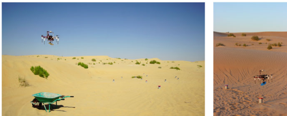
FIGURE 16 Photos from the tests of the proposed system in the desert near Abu Dhabi, United Arab Emirates. The grasping procedure is captured in the image on the right, and the dropping maneuver is shown in the image on the left. http://mrs.felk.cvut.cz/jfr2018treasurehunt-video3 [Color figure can be viewed at wileyonlinelibrary.com]
