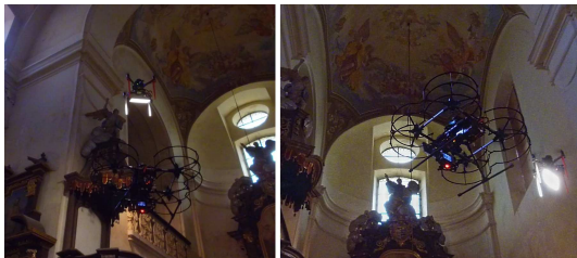
Fig. 2: Deployment of the proposed system for autonomous RTI by a team of UAVs in Church of St. Mary Magdalene in Chlumín. Multimedia material of the experiment is available at http://mrs.felk.cvut.cz/papers/rtri2020ral .
