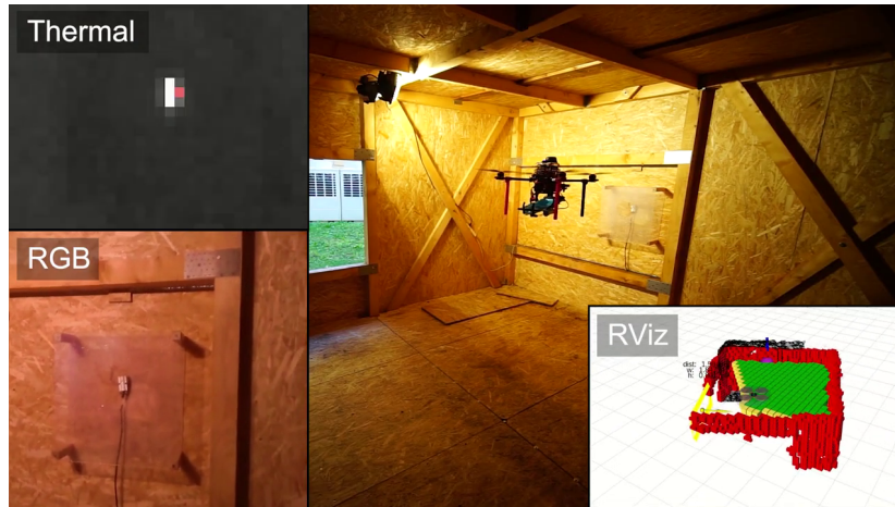
Figure 2.1: A photo of the fully autonomous UAV system developed for extinguishing fires inside buildings. The photo also shows the processed data from the onboard sensors of the UAV [1c].
