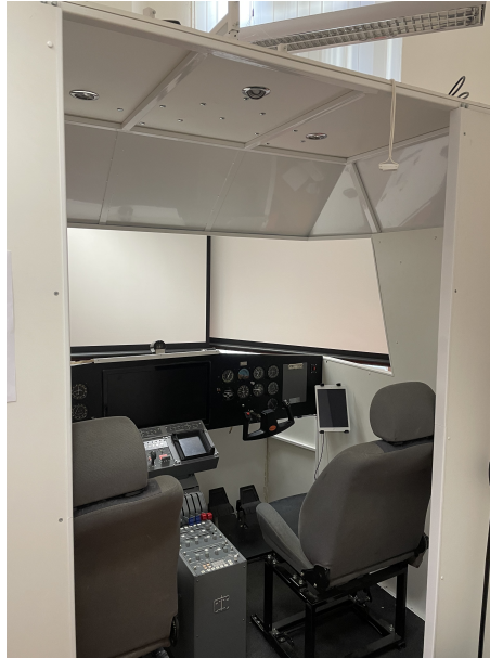
Figure 2.2: Multi-Engine Piston (MEP) Beechcraft Simulator of the Department of Air Transport (source: author's photograph)
