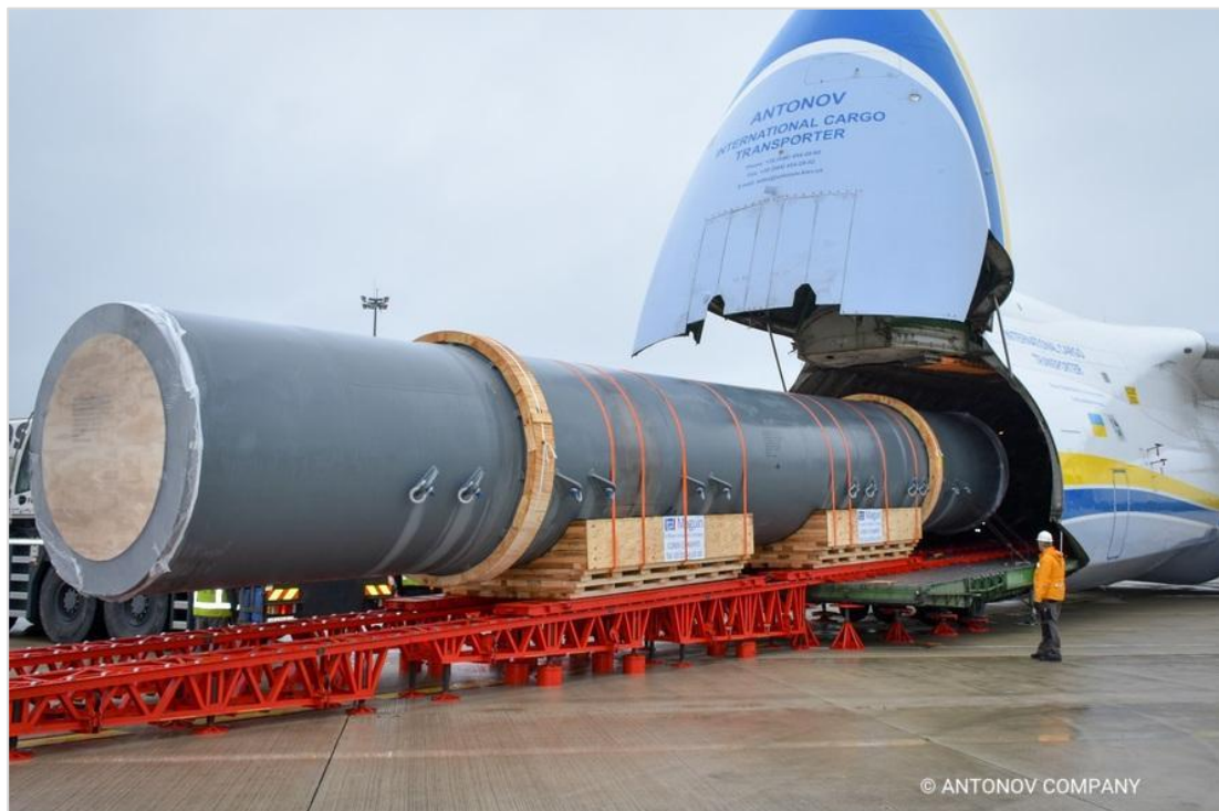
Figure 5, Loading of the mining equipment at Paris-Vatry Airport, Antonov An-225, [12].
