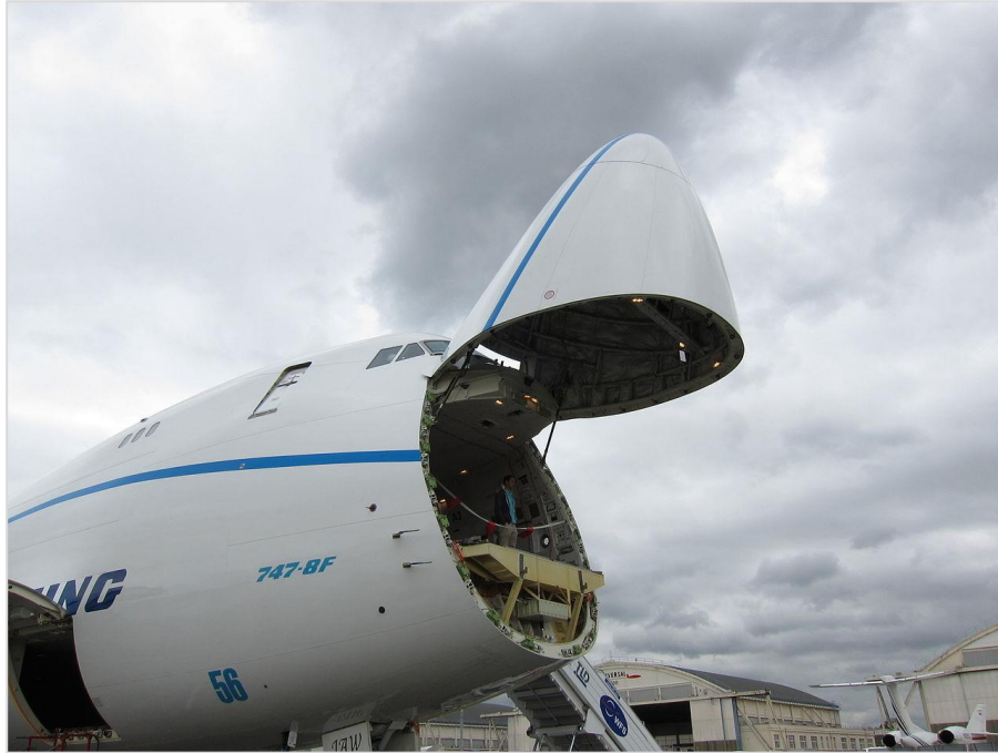
Figure 7, Nose Cargo Door of a Boeing 747-8f, Displayed at the 2011 Paris Air Show, [26].
