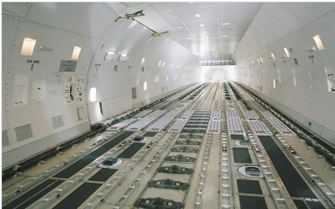
Figure 14, Main Deck of a Converted Boeing B747-400BDSF, [73].
