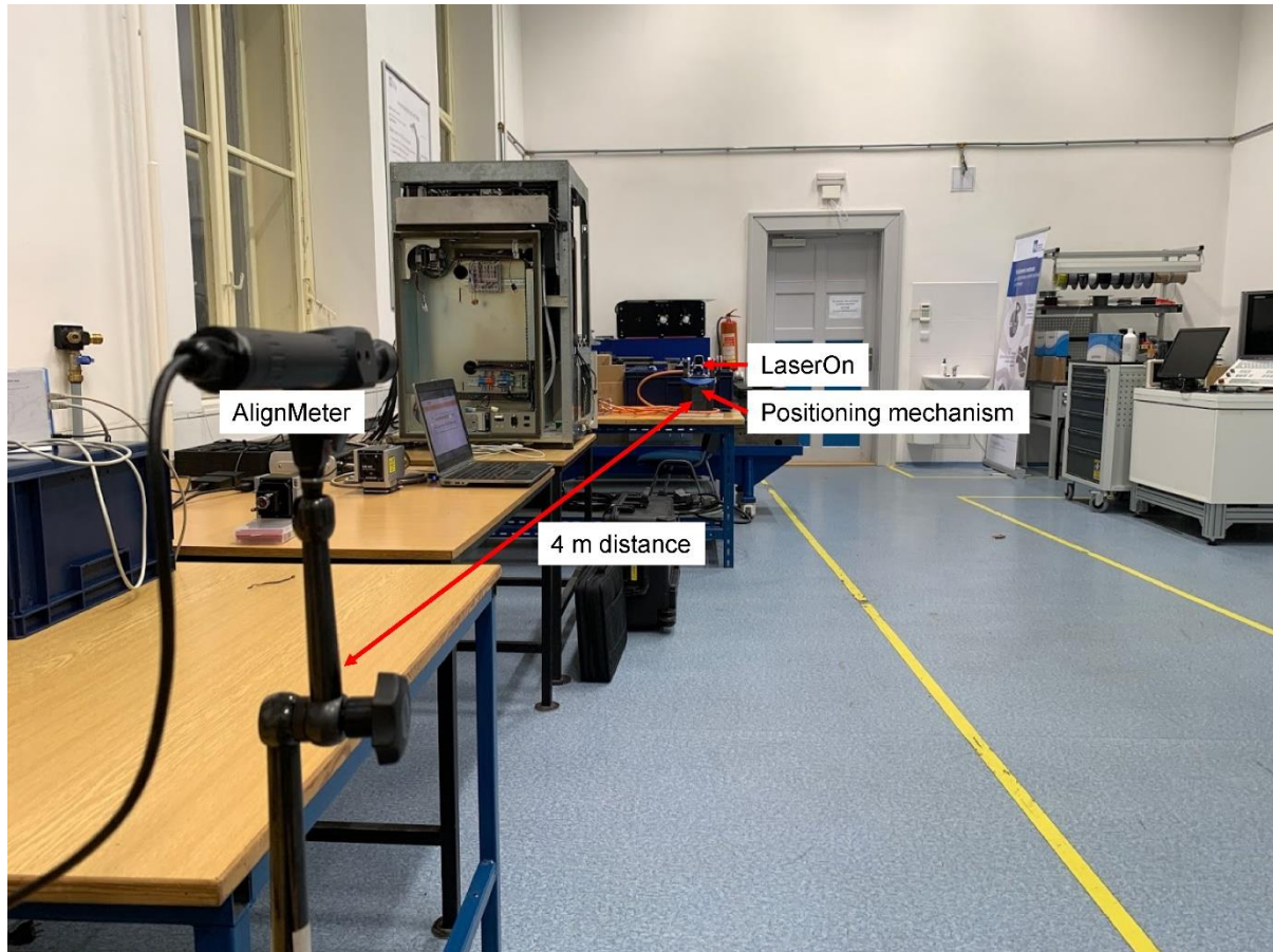
Fig. 58: Setup for preliminary testing of positioning resolution
