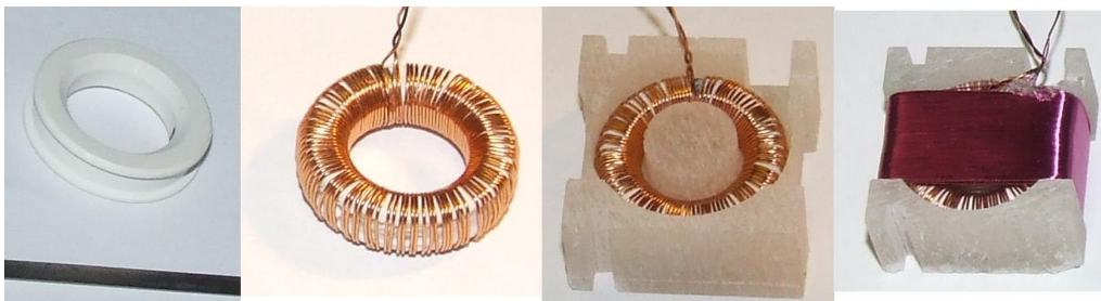
Fig. 3.8 From left to right: BNP-2 ring support and Vitrovac 6025X ribbon; the ring with glued core and excitation winding; placed in the pick-up coil support; finished sensor with pick-up coil.
