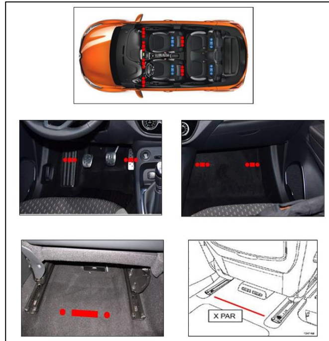
Figure 27 : thermal instrumentation in passenger compartment (Renault information)
