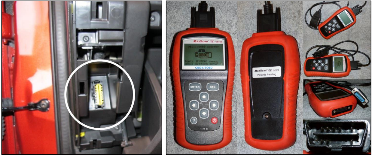
Figure 29 : OBD socket in Renault Kadjar and OBD reader (Wikipedia.en 2021)
