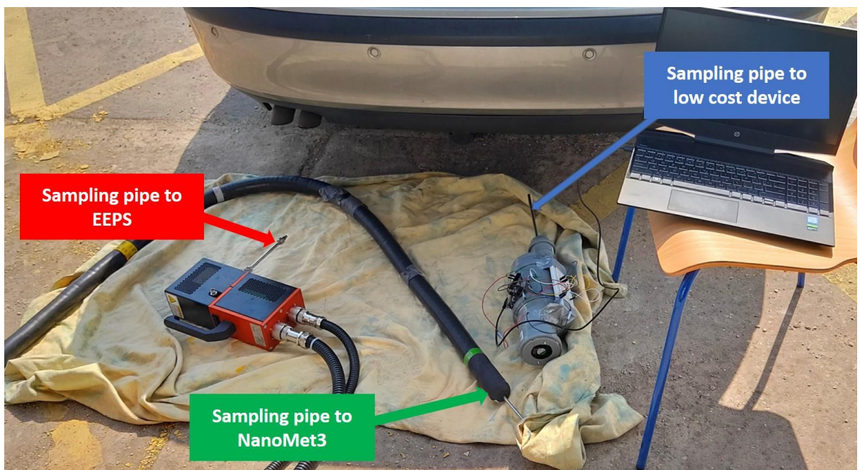
Figure 4.4-2 Sampling Pipe of Three Instruments
