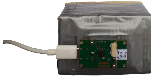
Figure 5.2. Experimental setup for static data acquisition of Epson M-G365PDF1.
