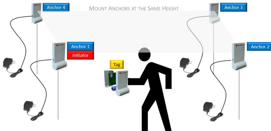
Figure 5.6. Positioning of UWB anchors and tags [42].
