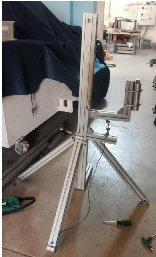
Fig. 14 - Measuring stand with attached motor
