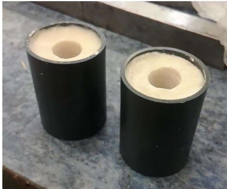
Fig. 13 - Finished BATES propellant grains
