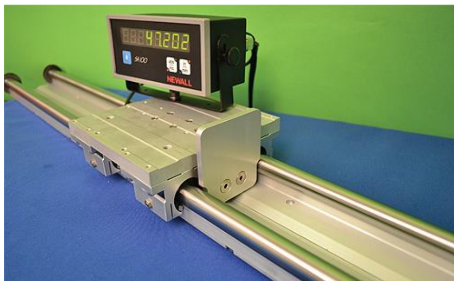
Fig. 49 - Example of a linear measuring system [22]
