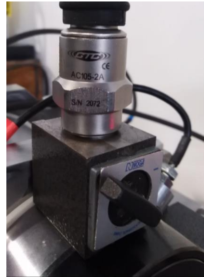
Figure 25. Measurement equipment: (a) NI-9234 input module [38] and (b) installed IEPE accelerometer
