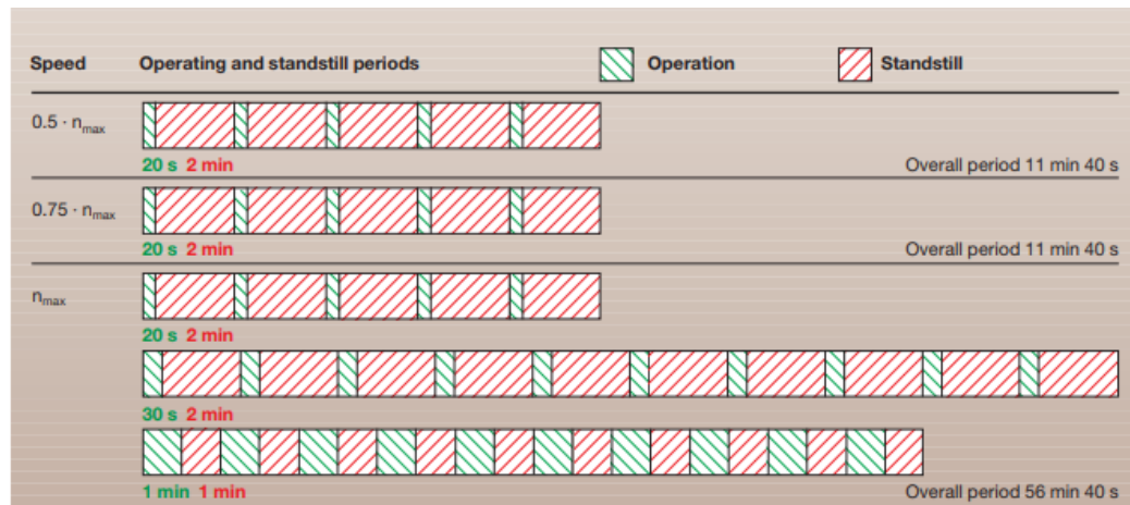
Figure 21. Grease distribution run procedure diagram [36]
