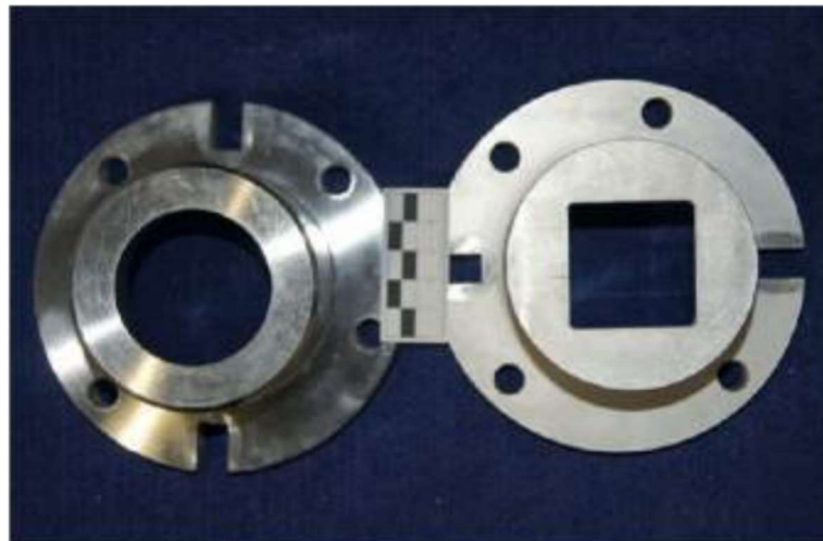
Figure 2-38: Mouthpieces for circular and square cross-sections [Kra15]
