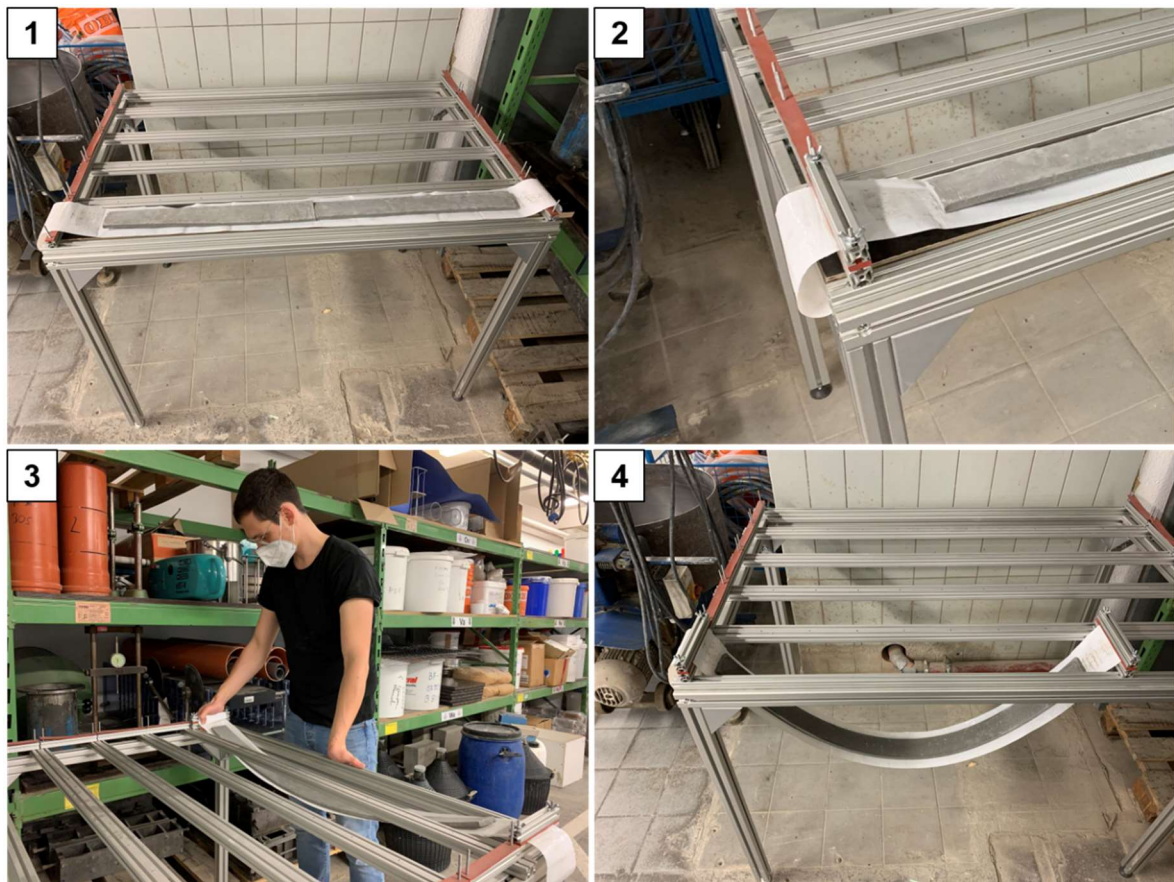
Figure 4-23: Steps of the longitudinal folding procedure
