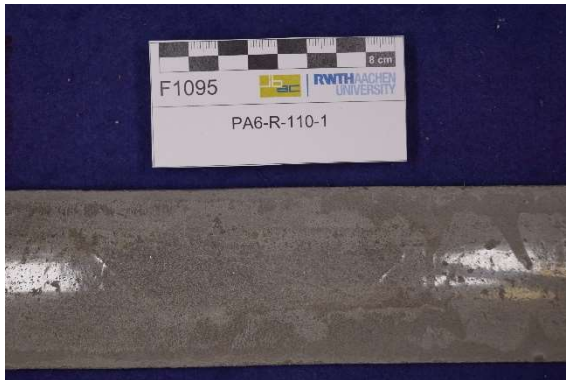
Figure A-10: Transversally formed concrete specimen without visible cracks (0.25 vol.-% of basalt fibers and no textile reinforcement) – bending radius approx. 5.1 cm
