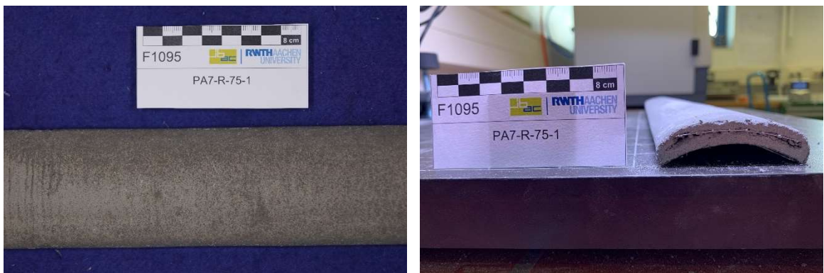
Figure A-15: Transversally formed concrete specimen without visible cracks (0.5 vol.-% of “soft” PVA fibers and ar-glass textile reinforcement) – bending radius approx. 5.3 cm
