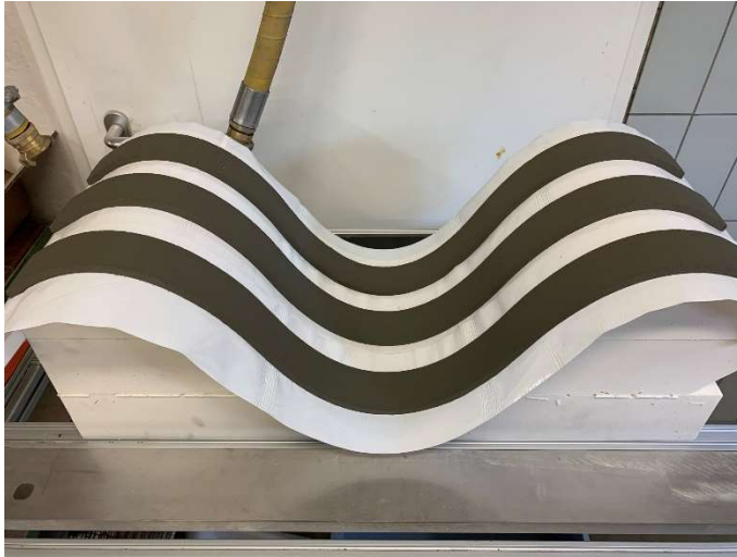
Figure 4-29: Double curved elements – fresh FRC (test series 5)
