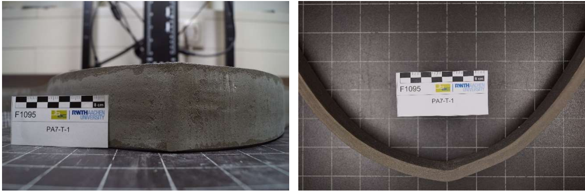
Figure 5-32: Double curved concrete specimens with kink (0.5 vol.-% of “soft” PVA fibers and ar-glass textile reinforcement) – bending radius of the intermediate curvature approx. 11.2 cm
