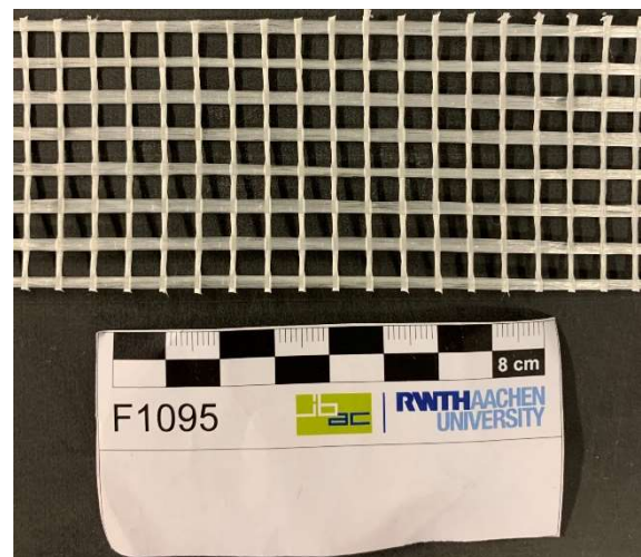
Figure 4-2: Textile reinforcement fabric used within this master’s thesis made from ar-glass
