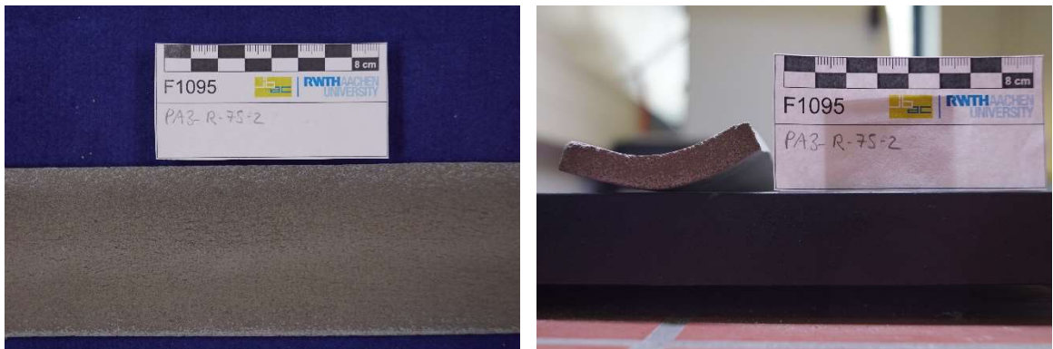
Figure A-14: Transversally formed concrete specimen with visible cracks of approx. 0.2 mm (0.5 vol.-% of basalt fibers and no textile reinforcement) – bending radius approx. 4.8 cm
