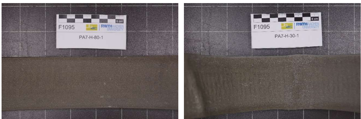
Figure A-19: Comparison of cross-section failures caused by longitudinal forming (concrete mixture with 0.5 vol.-% of “soft” PVA fibers and carbon textile reinforcement)
