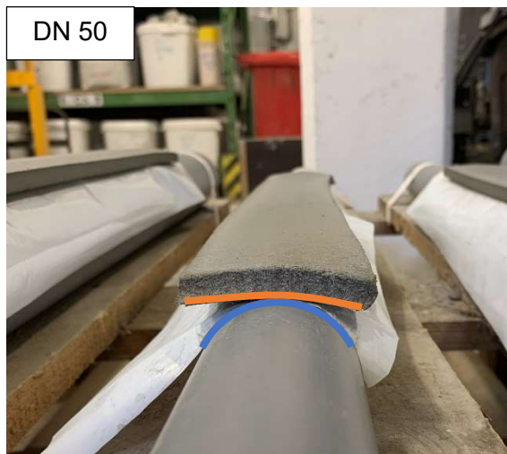
Figure 4-17: Transversally formed FRC on top of DN 50 pipe – free deformation (0.5 vol.-% of ‘soft’ PVA fibers and no textile reinforcement)
