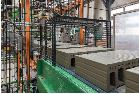
Figure 2-31: Brick production from endless extruded string [Zie21]
