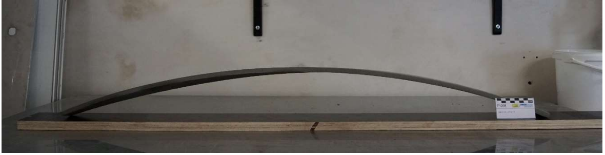
Figure A-6: Twisted longitudinally formed specimen (0.5 vol.-% of "hard" PVA fibers and no textile reinforcement)
