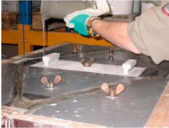
Figure 2-10: Casting a diamond shaped TRC element [Bra16]
