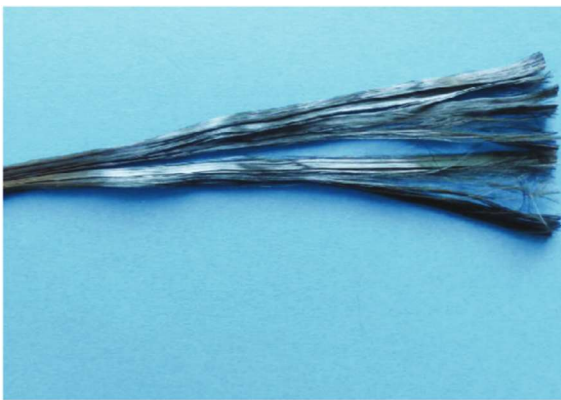
Figure 2-4: Multifilament roving made from carbon fibers [Rem18]
