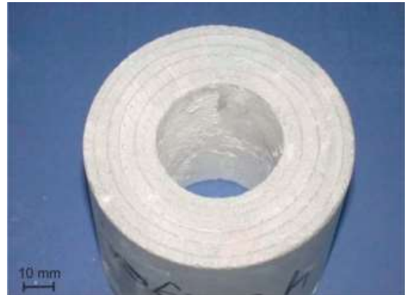
Figure 2-14: Spun tube with four layers of textile reinforcement [Bra16]
