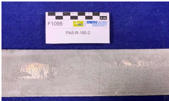
Figure A-8: Transversally formed concrete specimen without visible cracks (0.25 vol.-% of "soft" PVA fibers and no textile reinforcement) – bending radius approx. 7.2 cm
