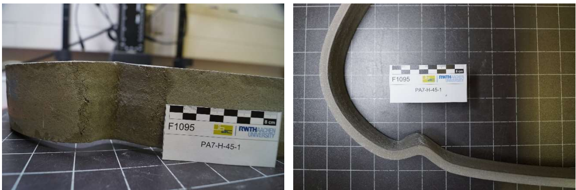
Figure A-21: Longitudinally formed concrete specimen without cracks (0.5 vol.-% of “soft” PVA fibers and ar-glass textile reinforcement) – bending radius undetermined
