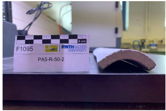
Figure A-9: Transversally formed concrete specimen with visible cracks of approx. 0.3 mm (0.25 vol.-% of “soft” PVA fibers and no textile reinforcement) – bending radius approx. 3.4 cm
