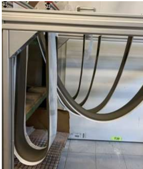
Figure 5-10: Vertical hanging concrete specimen without slipping (no fibers and no textile reinforcement)
