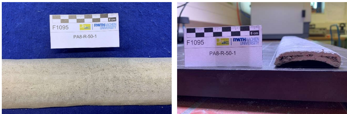
Figure 5-23: Transversally formed concrete specimen without visible cracks (0.5 vol.-% of "soft" PVA fibers and carbon textile reinforcement) – bending radius approx. 5.0 cm
