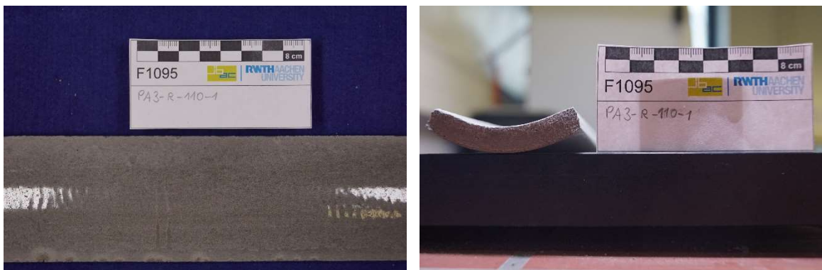
Figure 5-18: Transversally formed concrete specimen without visible cracks (0.5 vol.-% of basalt fibers and no textile reinforcement) – bending radius approx. 5.6 cm
