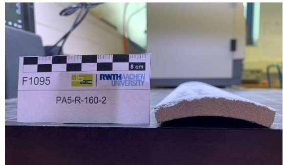
Figure A-8: Transversally formed concrete specimen without visible cracks (0.25 vol.-% of "soft" PVA fibers and no textile reinforcement) – bending radius approx. 7.2 cm
