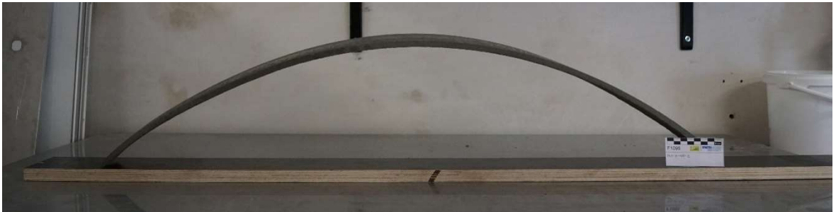
Figure A-7: Twisted longitudinally formed specimen (0.5 vol.-% of "hard" PVA fibers and no textile reinforcement)
