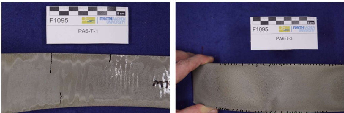
Figure 5-31: Double curved concrete specimens with visible cracks (0.25 vol.-% of basalt fibers and no textile reinforcement) – bending radius of the intermediate curvature on average 11.6 cm
