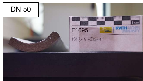
Figure 4-21: Transversally formed FRC– forced deformation (0.5 vol.-% of basalt fibers and no textile reinforcement)
