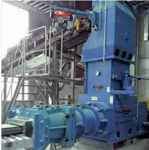
Figure 2-34: Industrial-scale extruder for fiber reinforced cement-bound material by Händle GmbH [Hän19]
