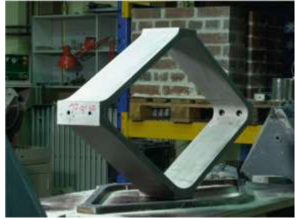
Figure 2-11: Finished cast TRC element for a lattice arch [Bra16]
