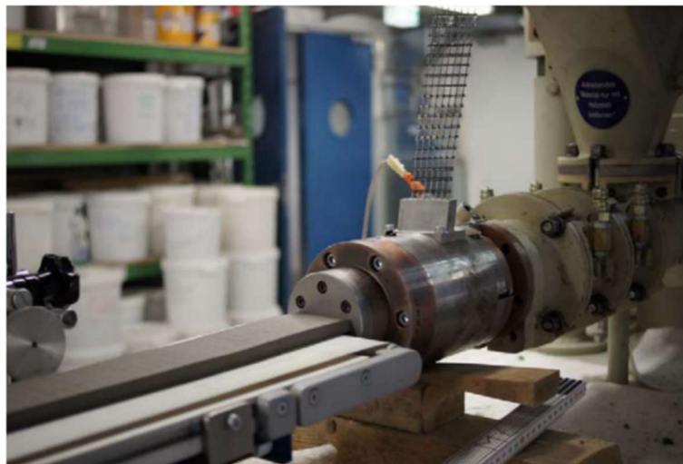
Figure 2-42: Extrusion with feeding device for fabrics [Bra15]
