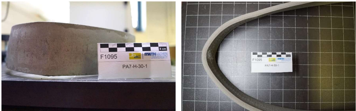
Figure A-18: Longitudinally formed concrete specimen with kink and buckling (0.5 vol.-% of “soft” PVA fibers and ar-glass textile reinforcement) – bending radius undetermined
