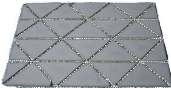
Figure 2-25: Oricrete-plate with Yoshimura crease pattern [Woe13]
