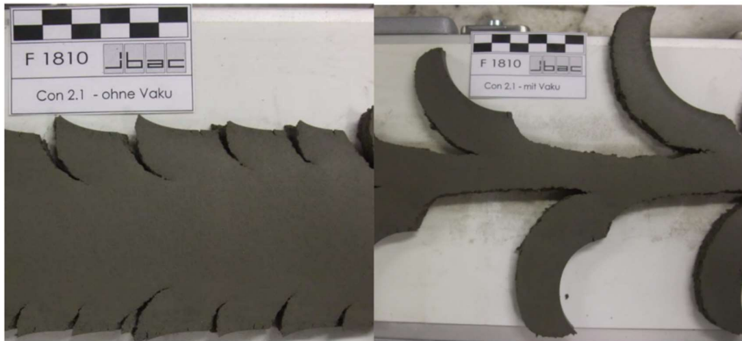
Figure 2-37: Results of extrusion with unsuitable concrete mixtures – Left: no vacuum applied Right: vacuum applied [Bra15]
