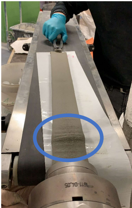
Figure 4-11: Pulling on the textile fabric – Concrete piling up on transverse rovings
