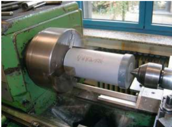
Figure 2-13: Clamped tube during spinning process [Bra16]
