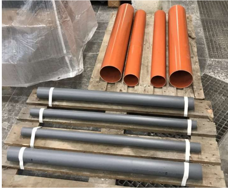
Figure 4-13: Pipes used for transverse folding of extruded concrete
