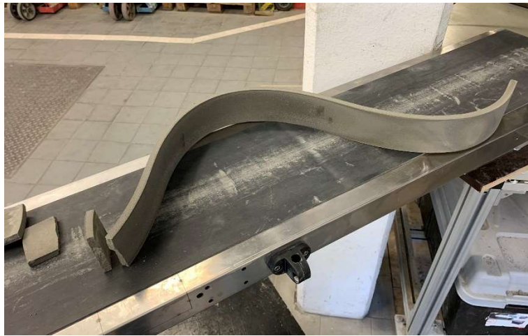
Figure A-23: Specimen failed after curing (0.25 vol.-% of basalt fibers and no textile reinforcement)
