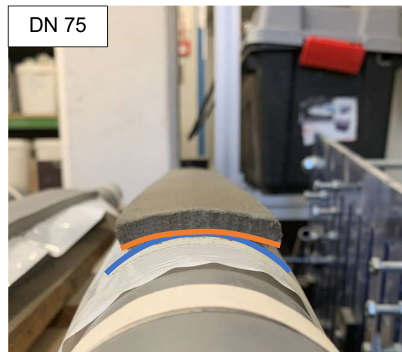
Figure 4-18: Transversally formed FRC on top of DN 75 pipe – free deformation (0.5 vol.-% of ‘soft’ PVA fibers and no textile reinforcement)
