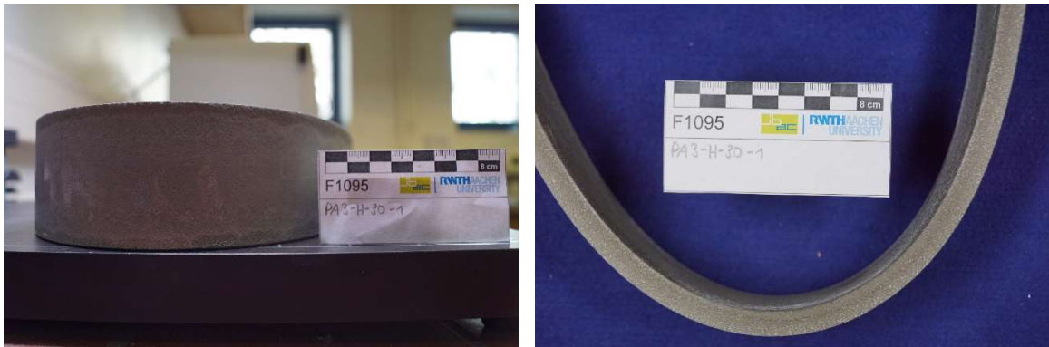
Figure 5-21: Longitudinally formed concrete specimen without cracks (0.5 vol.-% of basalt fibers and no textile reinforcement) – bending radius approx. 7.5 cm
