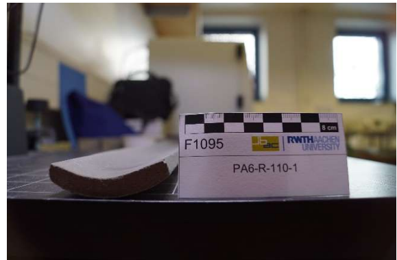
Figure A-10: Transversally formed concrete specimen without visible cracks (0.25 vol.-% of basalt fibers and no textile reinforcement) – bending radius approx. 5.1 cm
