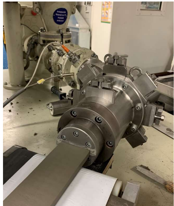
Figure 4-10: TRC specimen extruded with new mouthpiece
