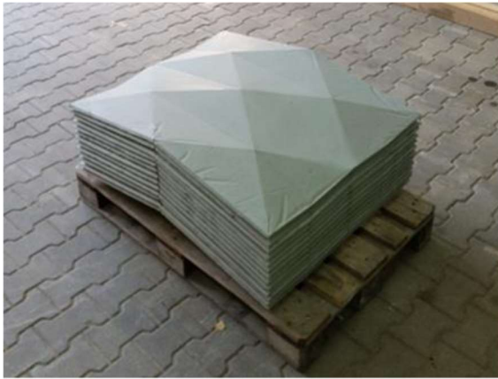
Figure 2-17: Folded segments produced by fold-in-fresh method [Woe17]
