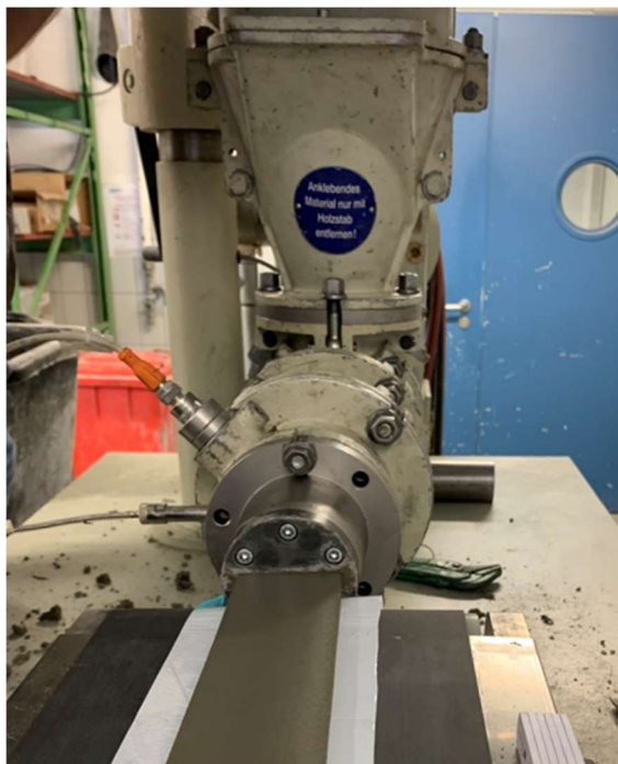
Figure 4-7: Extruded fine-grained concrete without textile reinforcement
