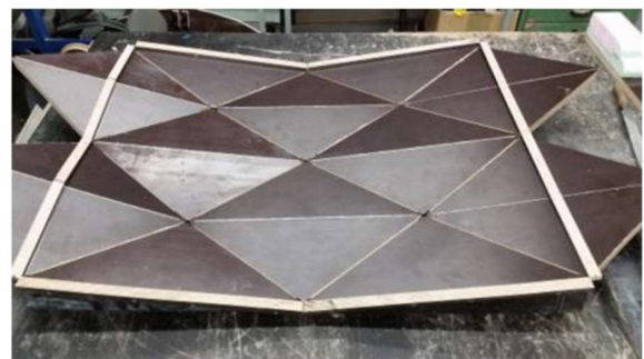
Figure 2-16: Foldable formwork in folded state [Woe17]
