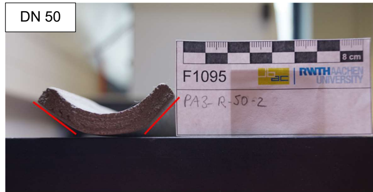
Figure 4-19: Edgy surface caused by roller pressure
