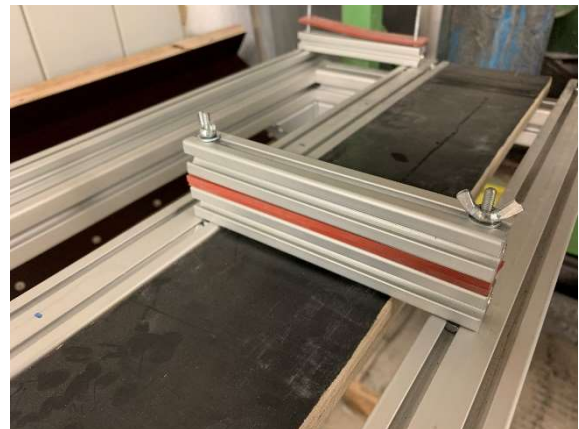
Figure 4-25: Structure of a clamping jaw - assembled
