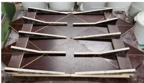
Figure 2-15: Components of a foldable formwork [Woe17]
