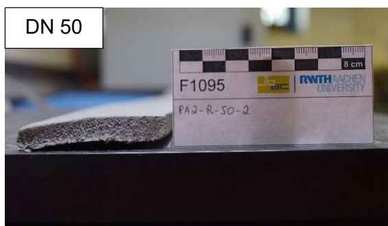
Figure 4-20: Transversally formed FRC– free deformation (0.5 vol.-% of “soft” PVA fibers and no textile reinforcement)
