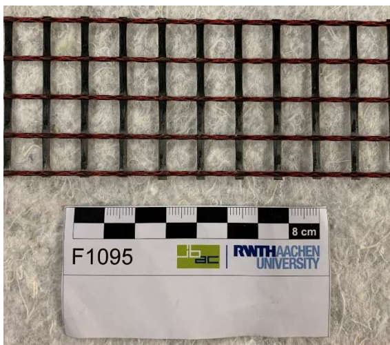
Figure 4-1: Textile reinforcement fabric used within this master’s thesis made from carbon
