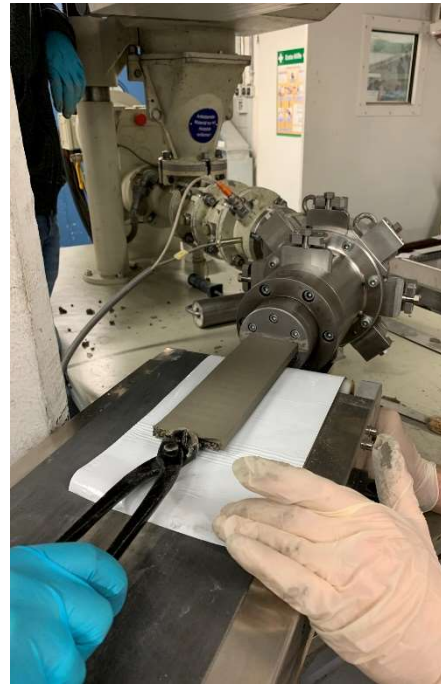
Figure 4-12: Pulling on the textile fabric – Extruded specimen without visible defects
