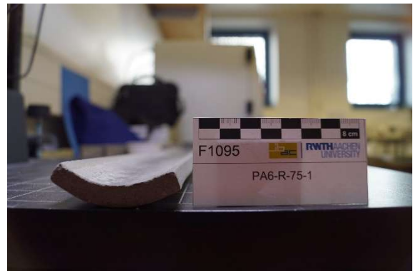
Figure A-11: Transversally formed concrete specimen with visible cracks of approx. 0.3 mm (0.25 vol.-% of basalt fibers and no textile reinforcement) – bending radius approx. 4.9 cm
