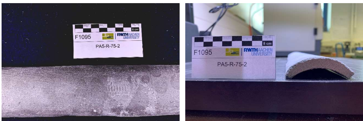
Figure 5-11: Transversally formed concrete specimen with visible cracks of approx. 0.2 mm (0.25 vol.-% of “soft” PVA fibers and no textile reinforcement) – bending radius approx. 4.5 cm
