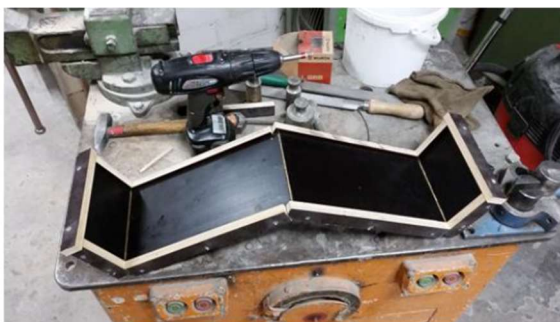
Figure 2-22: Formwork of specimen in folded configuration [Woe17]
