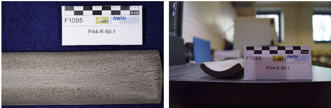
Figure 5-5: Transversally formed concrete specimen with visible cracks of approx. 0.4 mm (no fibers and no textile reinforcement) – bending radius approx. 3.8 cm
