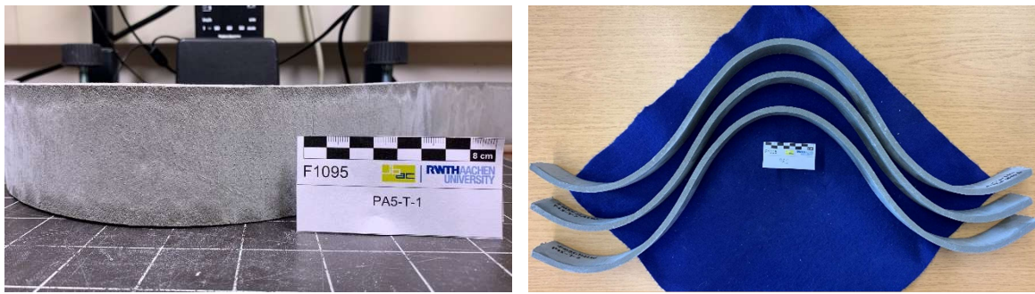
Figure 5-30: Double curved concrete specimens without visible cracks (0.25 vol.-% of “soft” PVA fibers and no textile reinforcement) – bending radius of the intermediate curvature on average 11.1 cm
