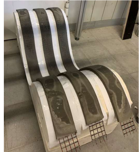
Figure 4-30: Double curved elements – cured TRC (test series 8)
