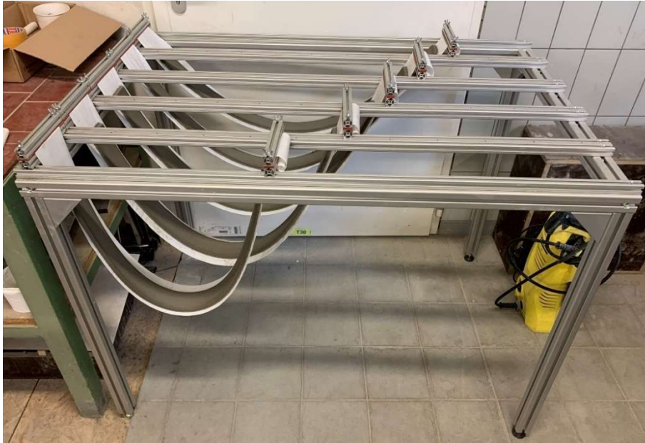
Figure 4-26: Test series 2 with longitudinally folded specimens
