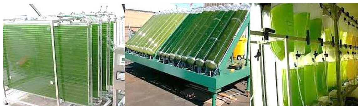
Figure 7 - Closed systems, from left: Flat panel PBR, Tubular PBR, and Bags system.
