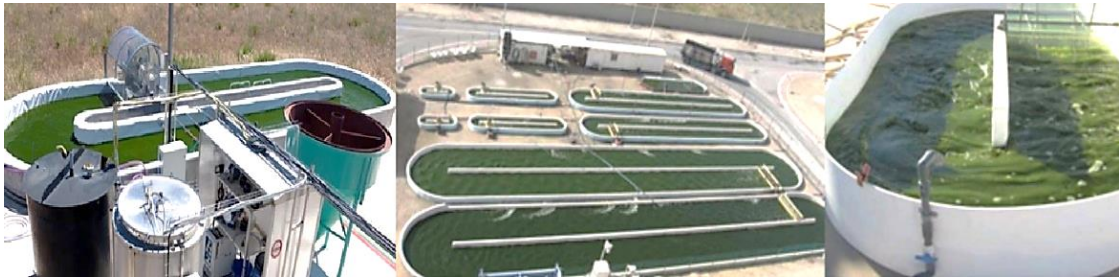
Figure 6 - Raceways system in different scale farms.
