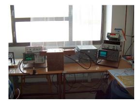
**Fig. 2** The working place for the measurement of nonlinearity of the I-V characteristics of the adhesive joints.
