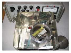
Fig. 4 The measurement of noise. Behind the screening box is the lock-in amplifier PAR 124 A.
