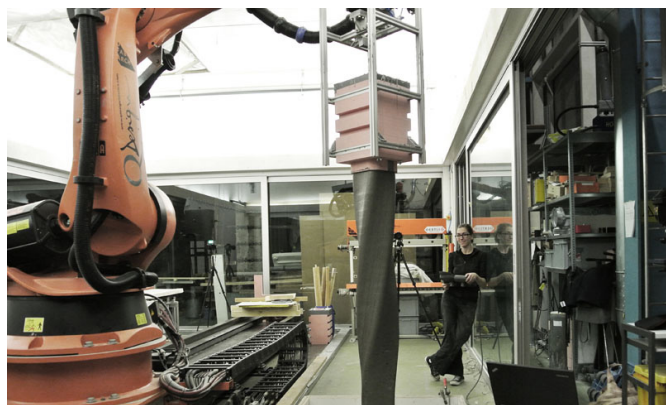
obr.120 Smart Dynamic Casting (2012-2015), Švajčiarsko, ETH Zürich [17.15]
