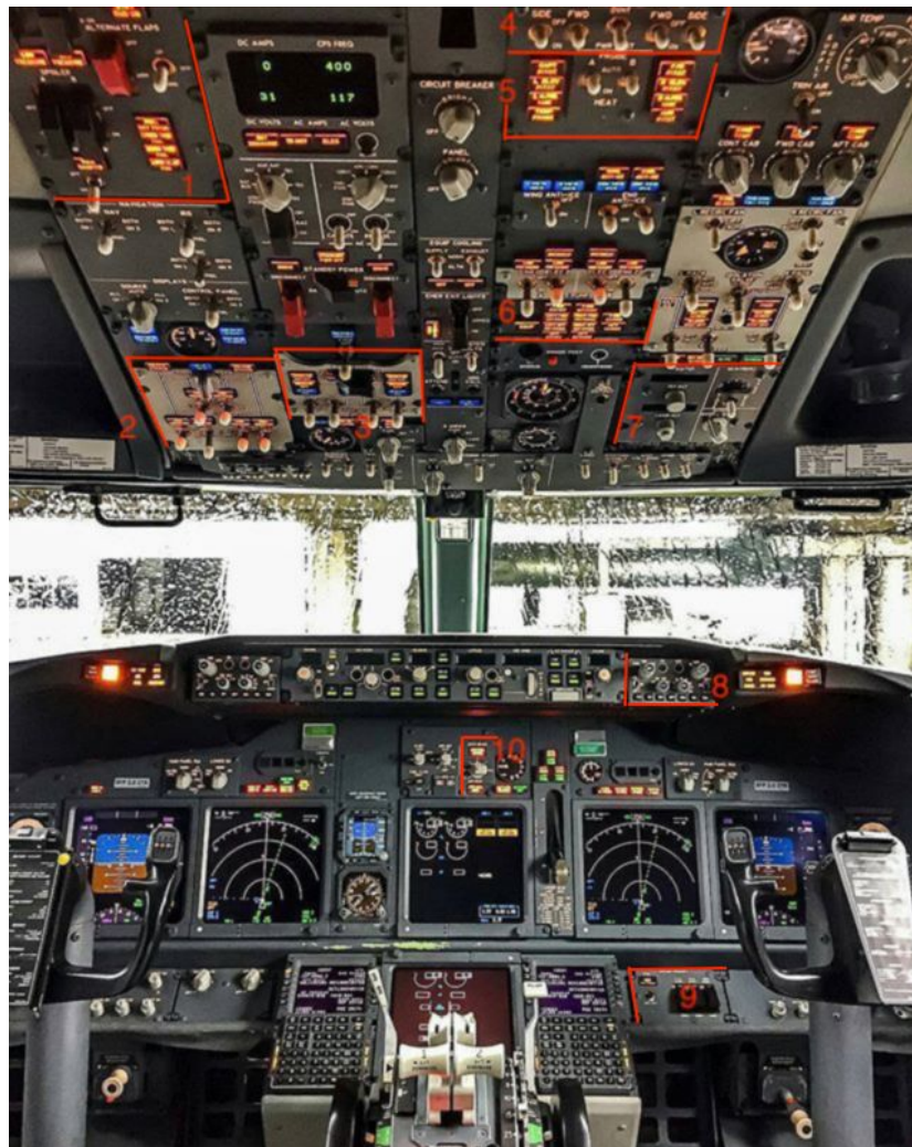
Obrázek 3.24: Kokpit letounu Boeing 737NG s označenými panely (1 - Flight control panel, 2 - Fuel panel, 3 - Electrical panel, 4 - Window heat panel, 5 - Probe heat panel, 6 - Hydraulic panel, 7 - Cabin pressurization panel, 8 - EFIS control panel, 9 - Ground proximity panel, 10 - Auto brake select switch)
