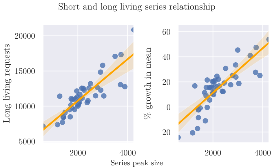
Figure 3.10: Figure explores the relationship of short and long-living series during peaks. The figure on the left compares the short-living series peak size with the requests in the long-living category measured simultaneously. The right figure compares the peak size with the percentual growth of long-living series during said peak over the mean measured at that time over the dataset.
