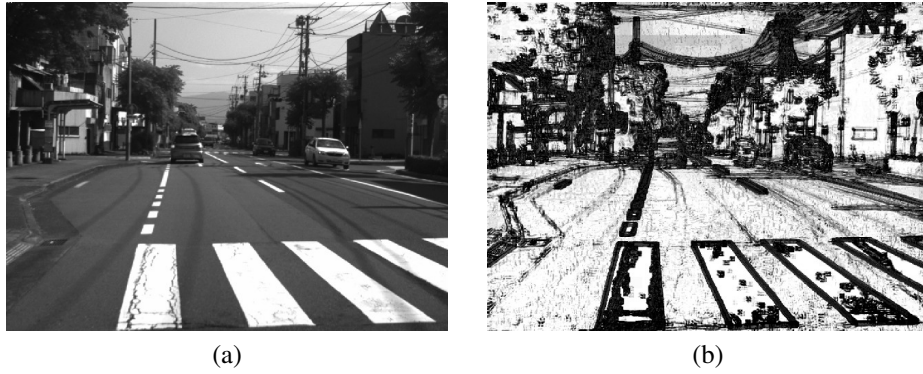
Figure 4. Coverage of an image by salient points. (a) A frame from an input video sequence. (b) Uniqueness of pixel descriptors within a search window. All pixels that are not white here are used for matching.
