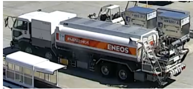
(b) Tank truck supplying fuel. Source: [14]
