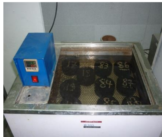
c) Submerging samples in water Figure 3. Moisture conditioning of the samples
