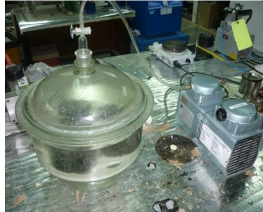
a) Vacuum saturation at room temperature
