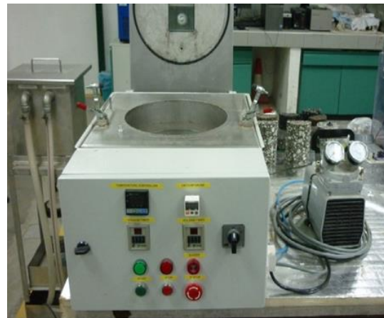
b) Vacuum saturation at 60°C
