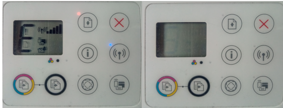
■ Figure 2.9 Device indicating error: flashing/blinking elements on control panel.
