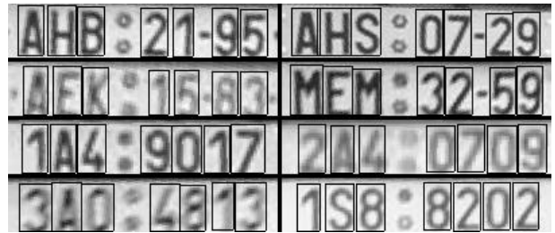
Fig. 7. Licence plate characters segmentation via CSER
