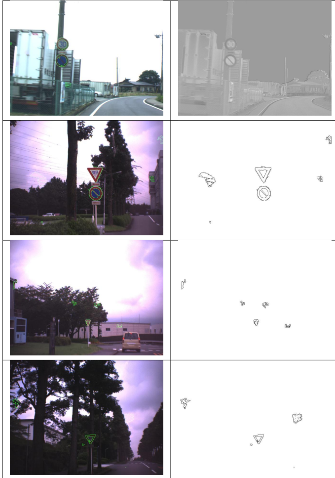
Fig. 8. Traffic signs detection results: First row shows traffic signs original image, then image thresholded in RB direction (i.e. from red to blue color) and detected regions. Other rows shows different images and the detected regions.
