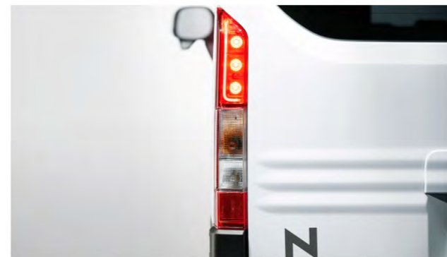
A rear combination lamp with an ultra-fine design that realizes a large-opening tailgate.
