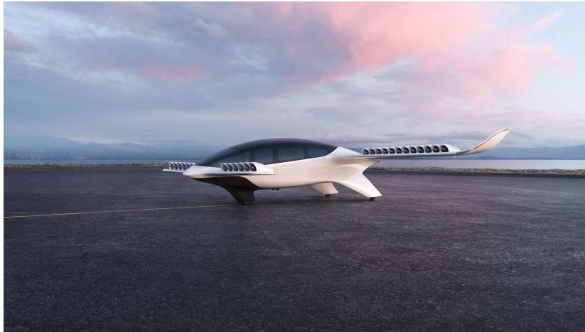
Figure 1.3: An electric VTOL aircraft being developed by Lilium. The technology has been successfully verified in-flight in 2019 on a 5-seater aircraft. A 7-seater model intended for production is currently being developed and certified by aviation authorities. The aircraft is expected to enter production in 2024. Credits: Lilium 3
