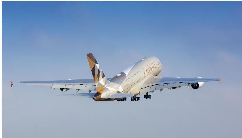
Figure 1.1: Airbus A380, the largest passenger aircraft in the world, in Etihad Airways livery during a take-off. The aircraft is 73 m long, 24 m high, and it has a wingspan of 80 m. Although the aircraft can carry up to 853 passengers, the typical capacity is 575 passengers. Credits: Airbus 1
