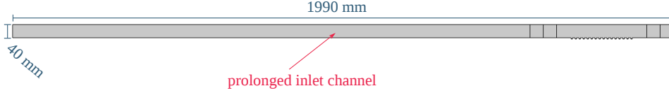
Figure 3.4: Geometry employed for the computation of the mean flow quantities.
