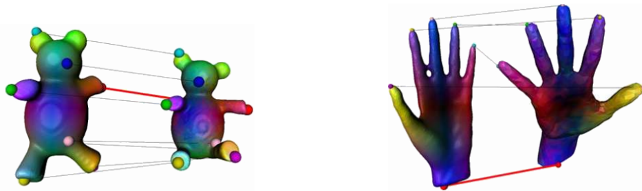
Figure 3.1: When evaluating vertex-to-vertex correspondence, either sparse or dense maps can be computed. Dense maps match all vertices between the two objects (illustrated by vertex color). With sparse maps, only a subset of all vertices is selected and matched instead (illustrated by points and lines). Image courtesy of [21] .
