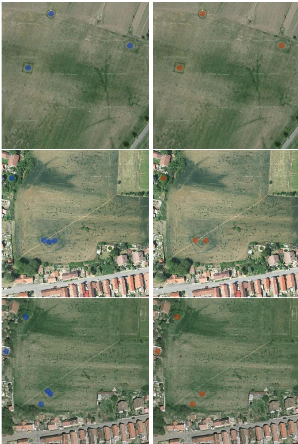
Figure F.13: GHT with circular templates: PC1 blob filtered dataset before (blue) and after (red) classification.
