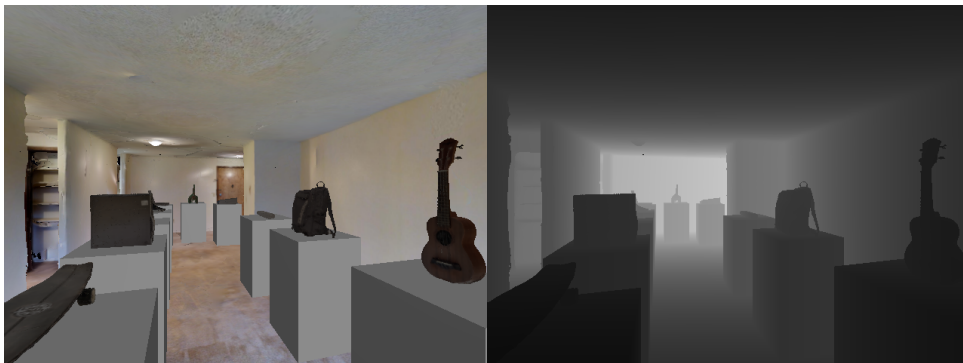
Figure 4.6: RGB and depth sensors inside Habitat simulation.
