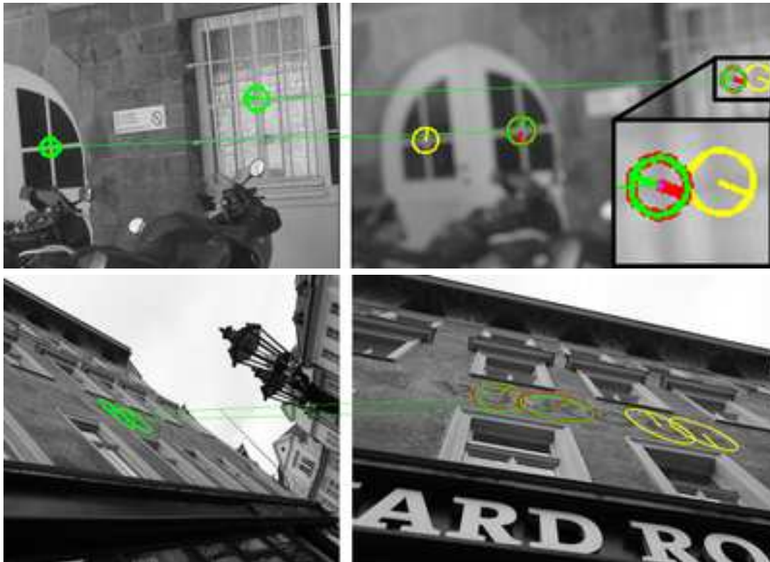
Figure 5.5: Green regions – correct correspondences rejected by the standard first to second closest ratio test (second closest region is in red), but recovered by the first to first geometrically inconsistent ratio (first geometrically inconsistent region is in yellow) matching strategy. DoG regions (top), MSERs (bottom).
