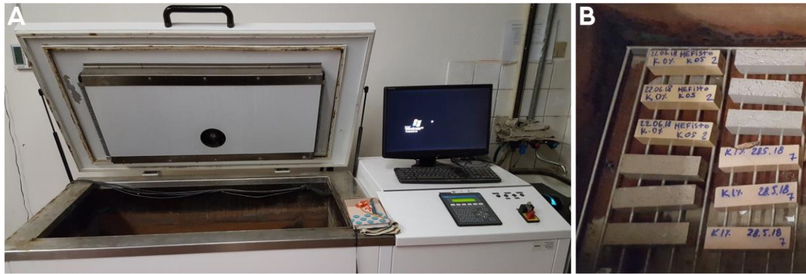
Fig. 20.: Frost resistance measuring freezer. (A) loading room, (B) sample arrangement
