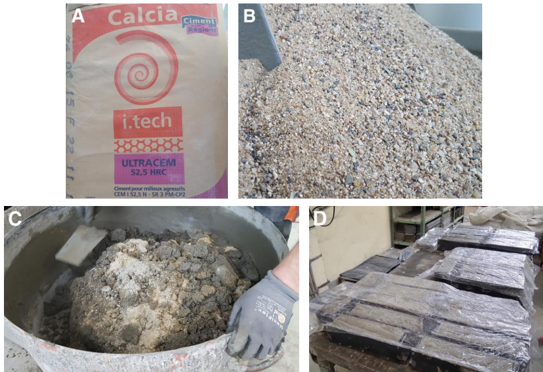
Fig. 12.: (A) Cement Calcias Ultracem 52,5 HRC, (B) Sand 0/4, (C) Mixing process, (D) Prepared samples covered with the PVC film
