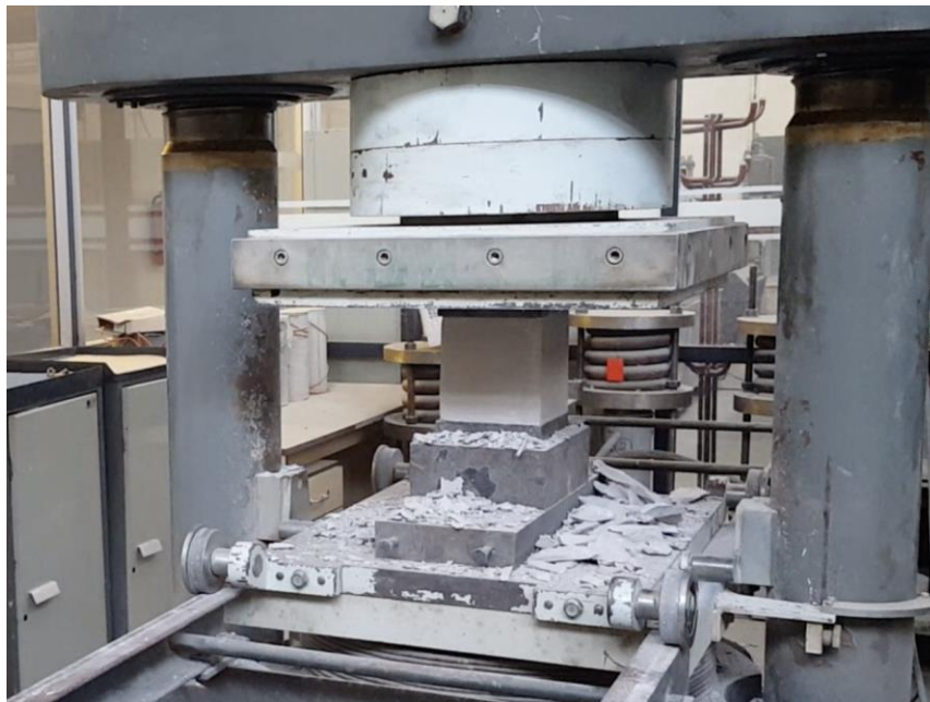
Fig. 14.: The 150 x 150 x 150 mm sample under the press load
