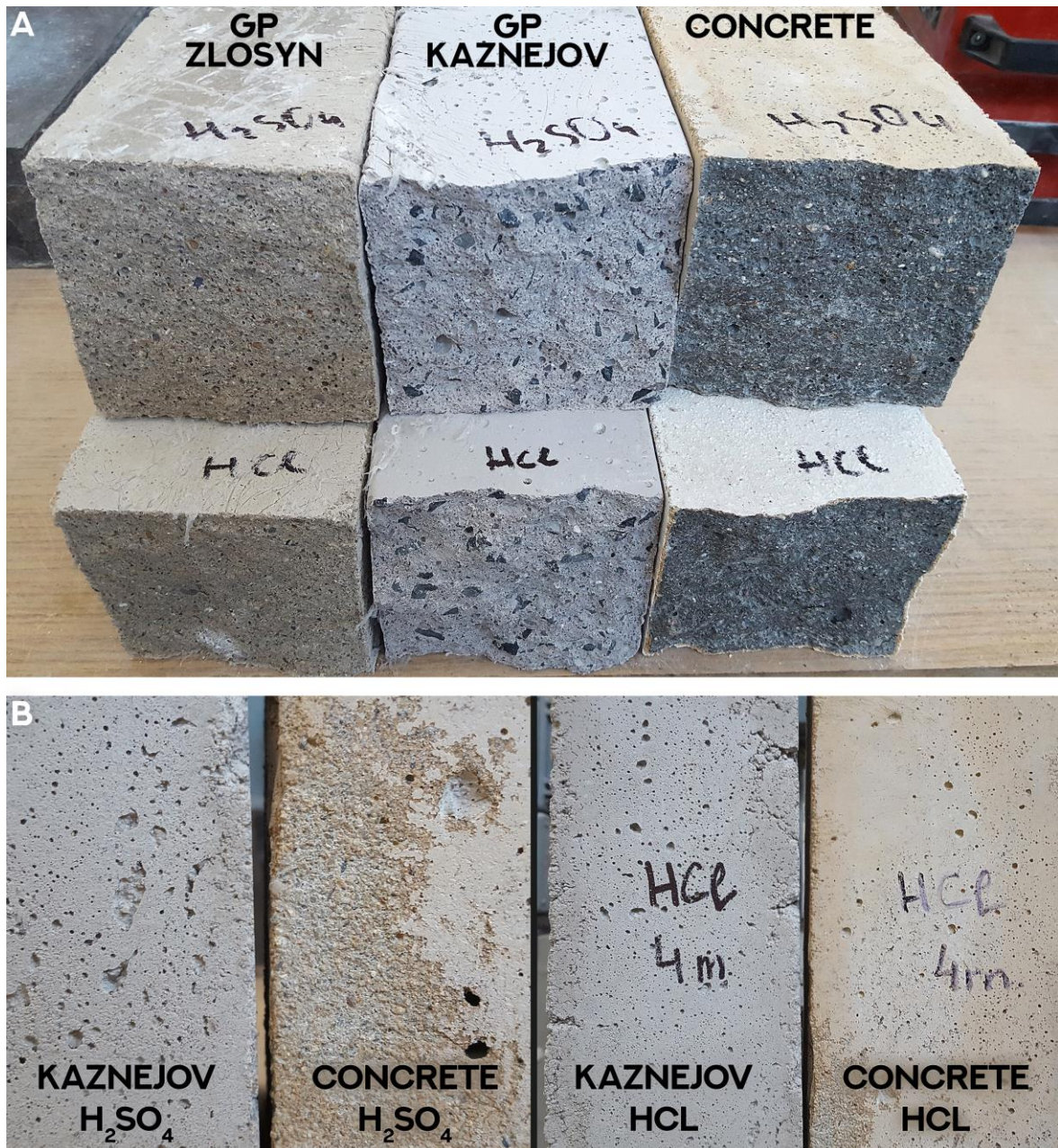
Fig. 41.: Visual comparison of geopolymer and concrete samples dried after 4 months in HCl and H_2SO_4 acids. (A) Photo of surface and inner structure of the samples, (B) detailed photo of dried samples' surface 4 month immersed in acids
