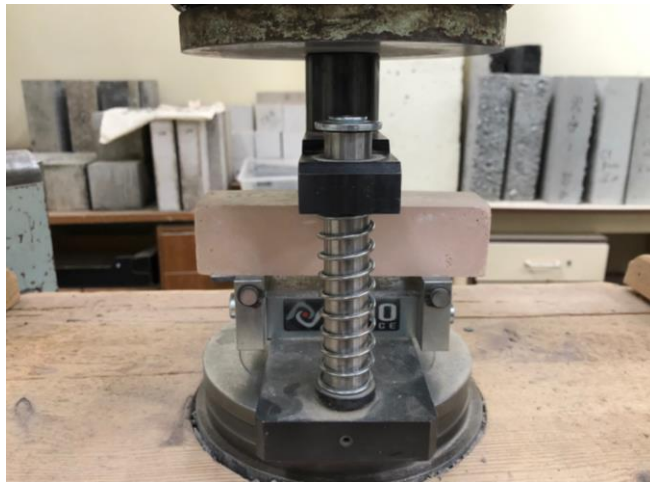
Fig. 15.: The 40 x 40 x 160 mm beam under the 3-point press load
