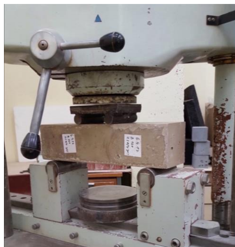
Fig. 16.: The 100 x 100 x 400 mm beam under the 4-point press load
