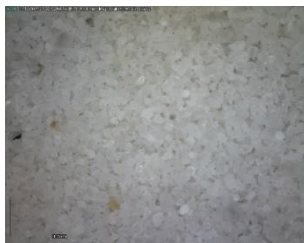
Figure 229- Střeleč quartz sand DinoLite microscope image, magnification 50
