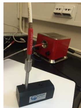
Figure 17 – White reference calibration (Spectralon)
