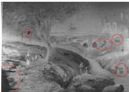
Figure 31 - IR image from SWIR VGA camera operating in 900 – 1700 nm spectral range with highlighted points that are not visible in the visible spectrum
