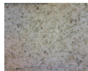
Figure 263 - Dolomite DinoLite microscope image, magnification 200
