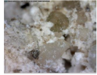
Figure 325 - Plaster sample 2 DinoLite microscope image, magnification 200
