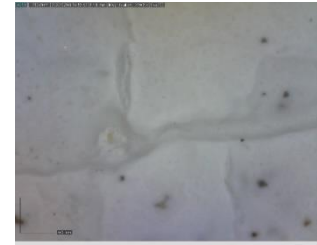
Figure 170 - Air lime mortar DinoLite microscope image, magnification 200
