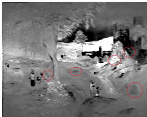
Figure 32 - Band 3 from principal component analysis with highlighted objects not visible on the original image
