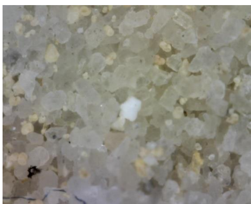
Figure 58 – Mšeno sandstone sample, DinoLite microscope image, Magnification 200
