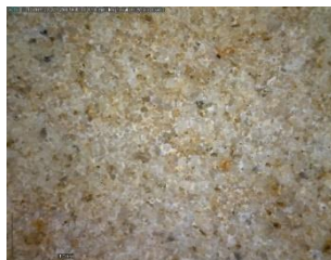
Figure 86 - Hořice sandstone DinoLite microscope image, magnification 50
