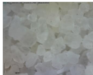
Figure 230 - Střeleč quartz sand DinoLite microscope image, magnification 200
