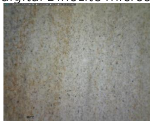
Figure 130 - Marlstone DinoLite microscope image, magnification 50
