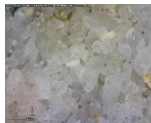
Figure 435 – Rock sample 1 - DinoLite microscope image, magnification 200
