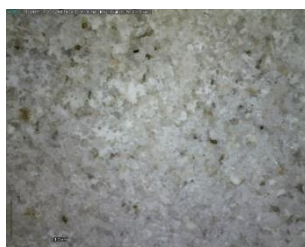
Figure 97 - Mšeno sandstone DinoLite microscope image, magnification 50
