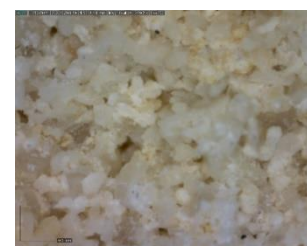
Figure 120 – Maastricht limestone DinoLite microscope image, magnification 200
