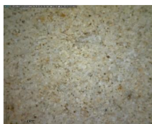
Figure 119 – Maastricht limestone DinoLite microscope image, magnification 50
