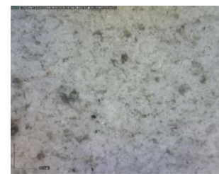
Figure 274 - Gypsum DinoLite microscope image, magnification 200
