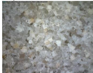
Figure 75 – Božanov sandstone DinoLite microscope image, magnification 50
