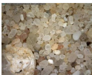
Figure 240 - Borek river sand DinoLite microscope image, magnification 50
