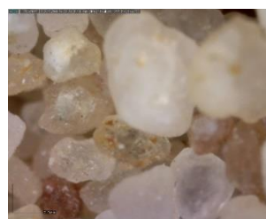
Figure 241 - Borek river sand DinoLite microscope image, magnification 200
