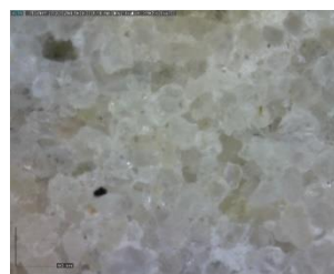
Figure 98 - Mšeno sandstone DinoLite microscope image, magnification 200
