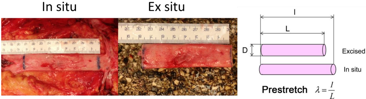
Figure 6. An evidence of the axial prestretch in abdominal aorta. Adopted from Horný et al. (2014).
