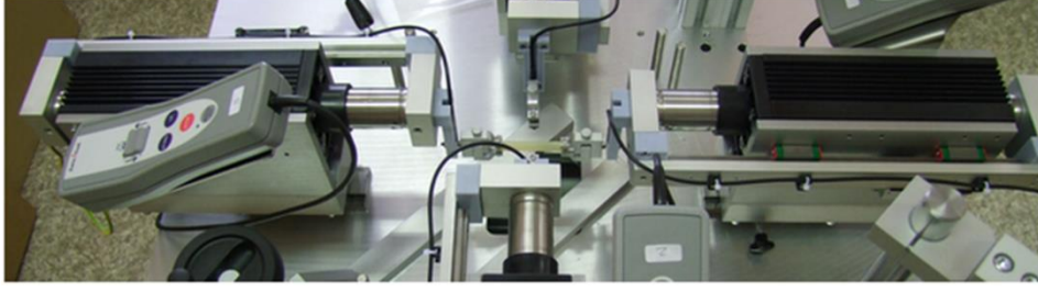
Figure 21. The multipurpose testing machine for uniaxial tensile test. Adopted from [Vonavkova et al., 2015].
