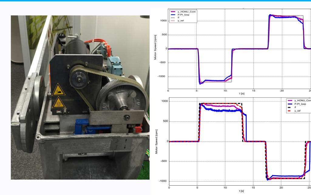
Optimization of cascade control loop with const. parameter HONU-MRAC control loop (QNU-QNU) via RLS(plant), GD(cont.) on real barrier drive control board. Barrier 1 (above) standard boom. Barrier 2 (below) with loaded boom. [10]
