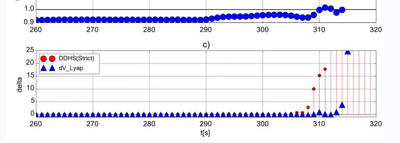
Comparative analysis of DDHS(Strict) with Lyapunov approach [4]-[5], [7]. Earlier detection via DDHS(Strict) of progressively unstable LNU-QNU control loop on conventional roller rig mathematical model.
