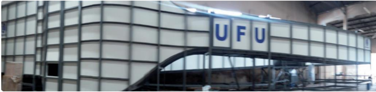
Figure 12. Steel frame and naval wood wind tunnel [21]
