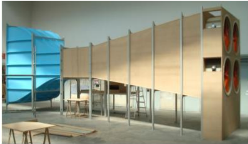
Figure 12. Steel frame and naval wood wind tunnel [21]
